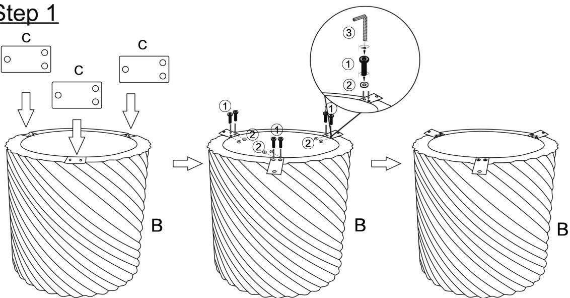
Open the carton, and place all the parts on a clean, non-marring surface. Take out Table Base(B). Align the holes of Connecting piece(C) with the holes of Table Base(B) as shown. Use Flat washer(②), Bolt(①) with Allen wrench(③) to tighten it.
