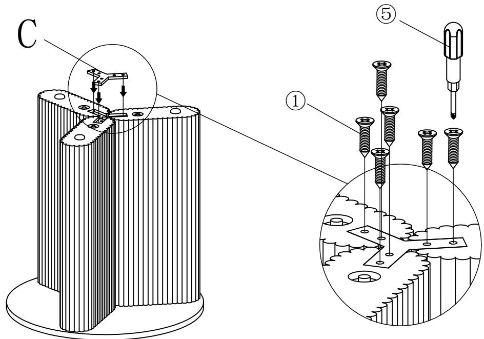
Attach the Connection Support(C) and Leg (B) use Bolt(①)with Phillips screwdriver(⑤).As shown above.
