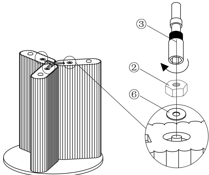
Use Sleeve(③) to secure the Leg(B) with Nut(②)and Washer(⑥) and table together. As shown above.
