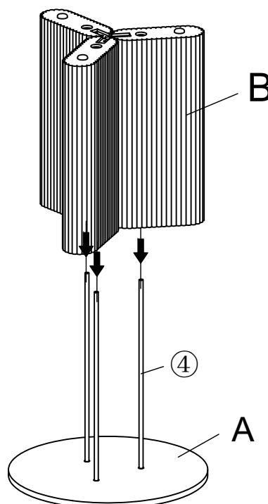
Attach the Table Top(A)to Leg(B), align Leg(B) with screw(④) hole position. As shown above.
