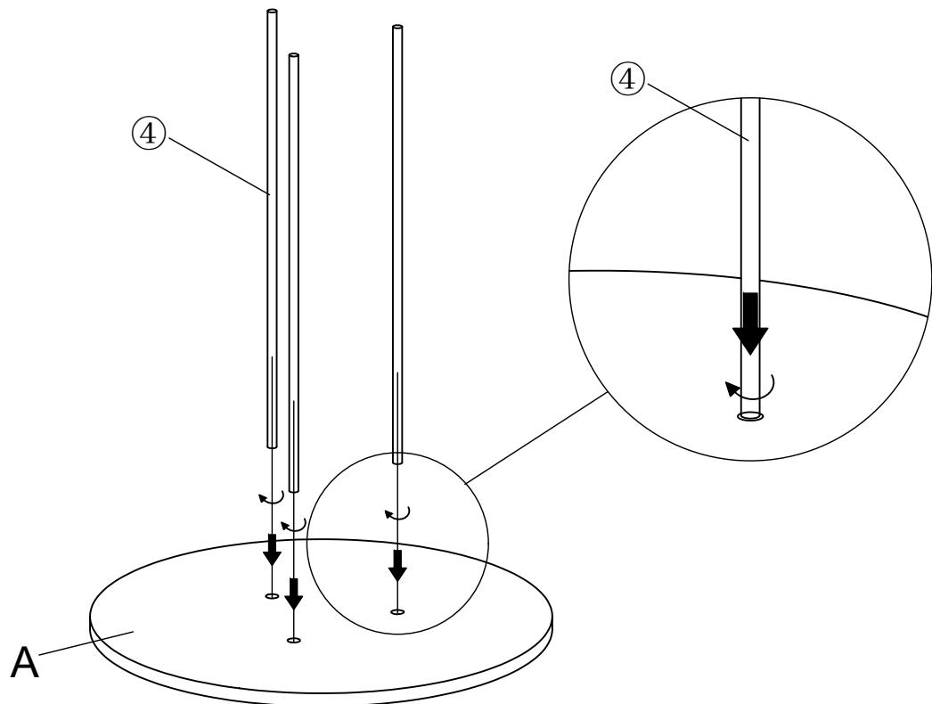
Attach the Table Top(A)to Leg(B)use Screw(4),Then tighten it.As shown above.
