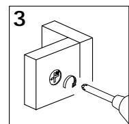
3: On the back of the Cam Lock will be a "C" shape. Insert the Cam Lock so the opening of the "C" fits over the Cam Bolt. Tighten with the screwdriver.
