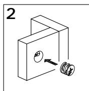
2: Fit the proper holes on the edge of the other part over the Cam Bolts. You should be able to see the cam bolts through the larger hole on the side.
