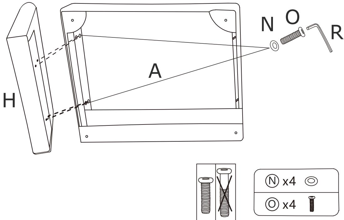
STEP 2: Assemble the Right armrest (I) to the Seat frame (A) with Washers (N) and Bolts (O).
