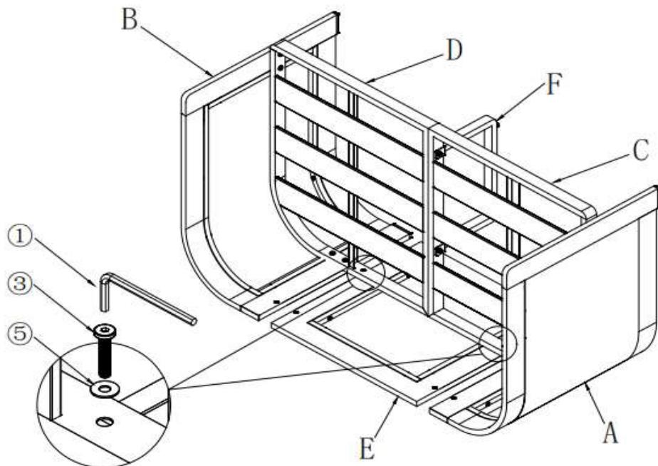
Attach the Seat (C & D) to Backrest Panel (E) using Bolts (③) and Washers (⑤) with Allen Wrench (①) as shown above.
