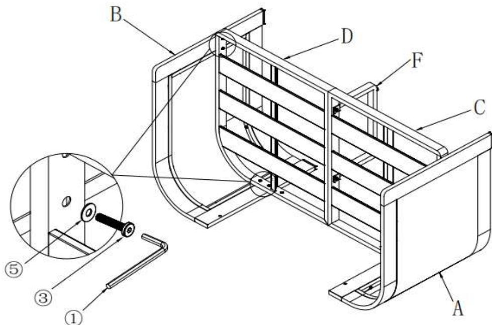
Attach the Right Seat (D) to the Right Armrest/Leg (B) using Bolts (③) and Washers (⑤) with Allen Wrench (①) as shown above.
