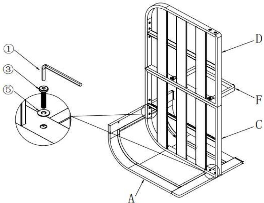
Attach the Left Seat (C) to the Left Armrest/Leg (A) using Bolts (③) and Washers (⑤) with Allen Wrench (①) as shown above.
