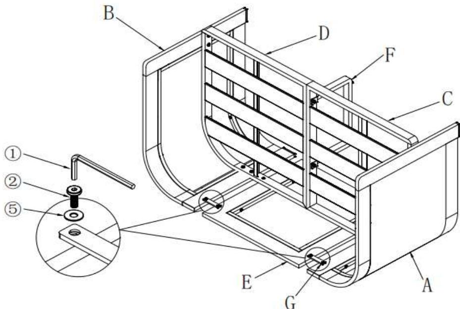
Connect the Backrest Panel (E) to the Armrests (A & B) with Connecting Washers (G), Bolts (②) and Washer(⑤) with Allen Wrench (①) as shown above.
