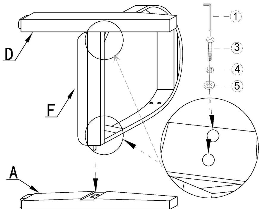
Install the Left Front Leg (A) and the Right Front Leg (D) onto the Seat cushion (F) connecting them via the Wooden Tenons (⑥), then using the Allen Wrench(①), Long Bolts(③), Spring Washers(④), and Flat Washers(⑤), attach them as shown in the picture above.
