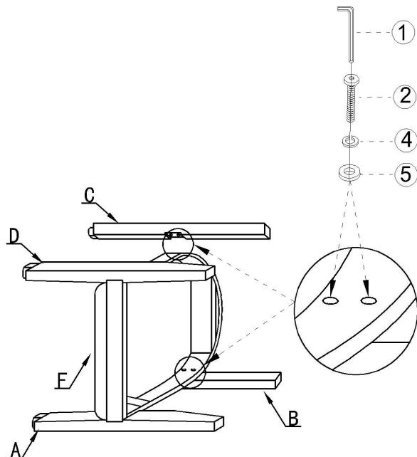
Install the Left Hind Leg(B) and Right Hind Leg(C) onto the Seat Cushion (F) using the Allen Wrench (①), Short Bolts(②), Spring Washers(④), and Flat Washers (⑤) as pictured above.
