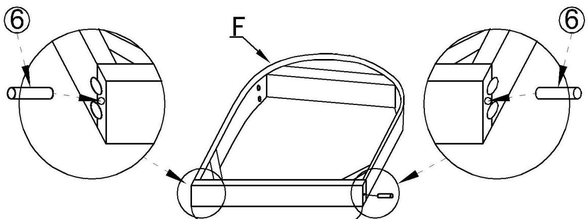
Install the Wooden Tenons(⑥) into the sides of the Seat cushion(F) as pictured above.
