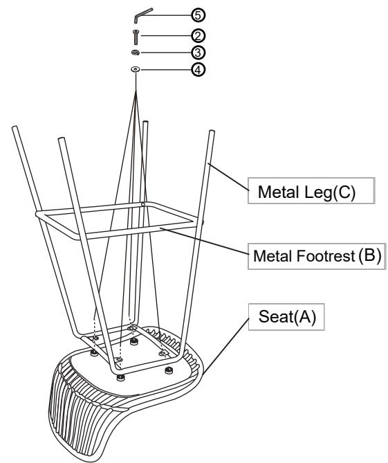
Place the Metal Leg (C) facedown, on a clean, non-marring surface. Put the Metal Footrest (B) into the Metal Leg (C), then attach the Metal Footrest (B) to Metal Leg (C) using Bolt(①) with Allen wrench( ④).
