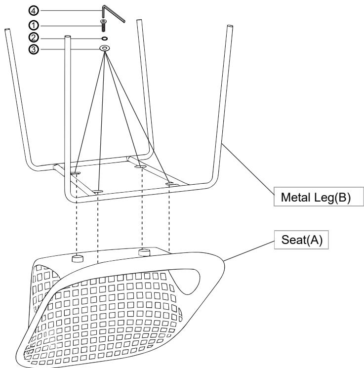
Place the Seat(A) facedown, on a clean, non-marring surface. Put the Metal Leg(B) into the Seat(A), then attach the metal Leg(B) to Seat(A) using Bolt(①), Spring Washer( ②), Flat Washer( ③) with Allen wrench( ④) .
