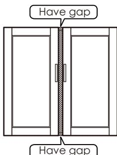
1 Turn "internal & external screw" to the right can make the door approach inside.
