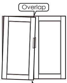
1 Turn "internal & external screw" to the left can make the top of the door tilted outward.
