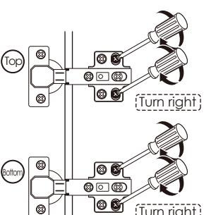
\* If the door is lower on bottom, please lift up the left door slightly on step 2
