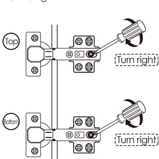
\* After adjusting the "front and rear screw", the door still does not change, please turn the "internal & external screw" to the right Slightly.
