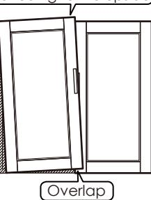
1 Turn "internal & external screw" to the left can make the bottom of the door tilted outward.
