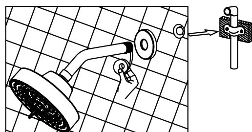
1. Install the shower arm, shower head, and flange to the fitting to the wall. Affix the shower head to the shower arm with the thread seal tape. (tape in the clockwise direction).
