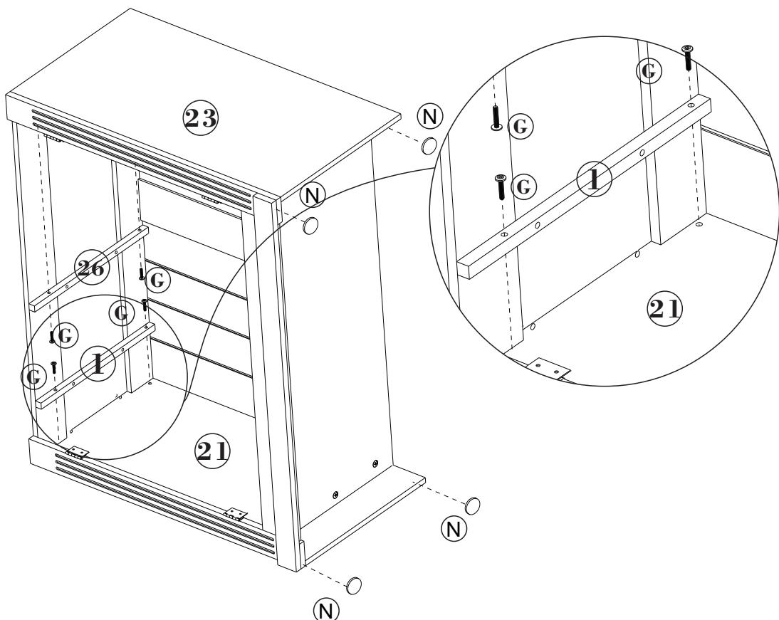
Don't fully tighten the G bolts to leave room for adjustment. Tighten them at last.
