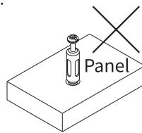
The pre-inserted nut should align with the center of the cam lock when joining two panels. The cam lock should be inserted before the eccentric wheel.
