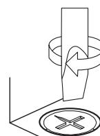
Turn the cam lock clockwise to tighten.
