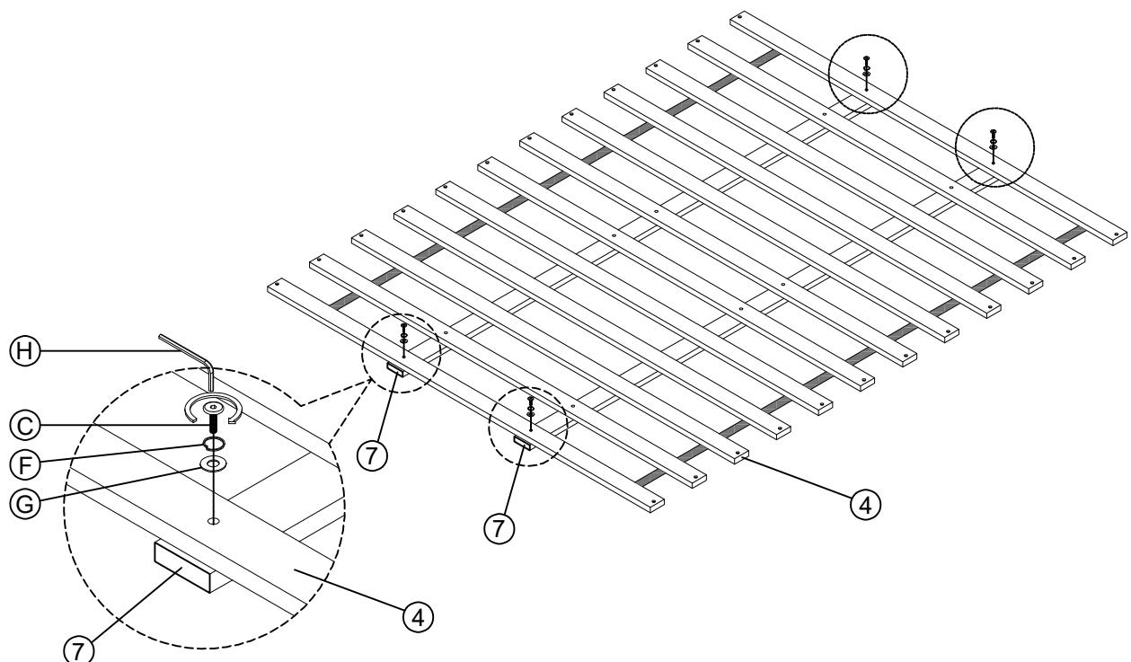
Assemble the Slat Roll (4) to Center Support Bar (7) using Bolts (C), Spring Washers (F), and Flat Washers (G). Tighten them with the Allen Wrench (H).
