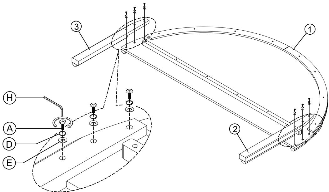
Assemble the Panel Headboard (1) to the Left Headboard Leg (2) and Right Headboard Leg (3) using Bolts (A), Spring Washers (D), and Flat Washers (E). Tighten them with the Allen Wrench (H) .
