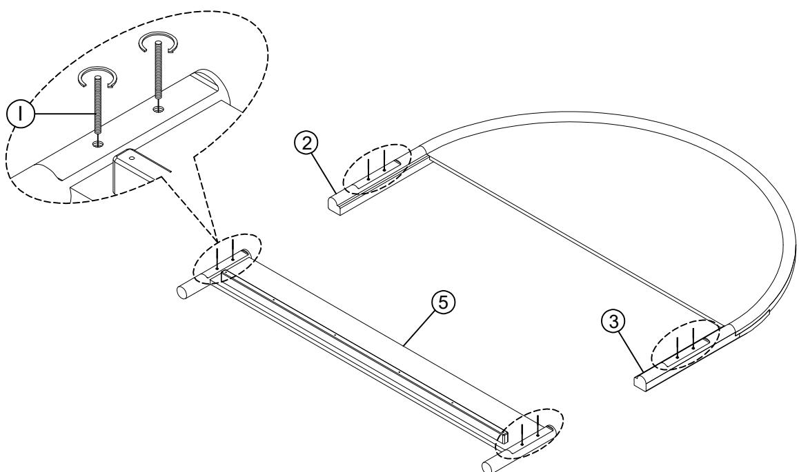
Attach the Hanger Bolts (I) to the Left Headboard Leg (2), Right Headboard Leg (3), and Footboard (5).
