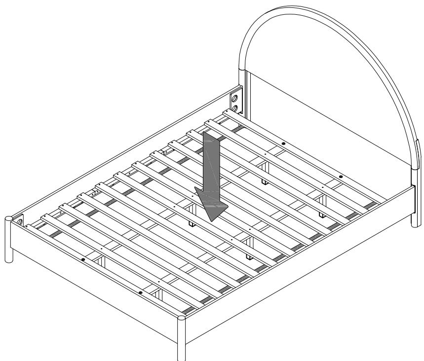
Place the assembled Slat Roll (4) Center Support Bar (7) and Support Leg (6) onto the Side Rails.
