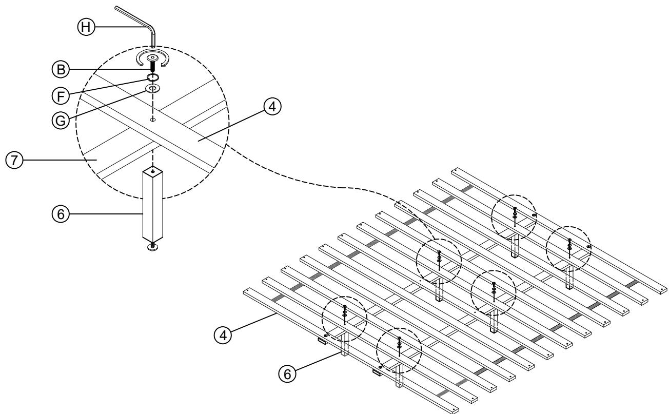
Attach the Support Leg (6) to the assembled Slat Roll (4) and Center Support Bar (7) using Bolts (B), Spring Washers (F), and Flat Washers (G). Tighten them with the Allen Wrench (H).
