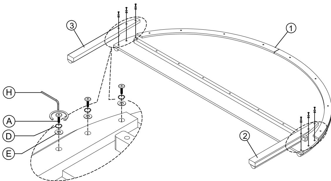
Assemble the Panel Headboard (1) to the Left Headboard Leg (2) and Right Headboard Leg (3) using Bolts (A), Spring Washers (D), and Flat Washers (E). Tighten them with the Allen Wrench (H) .
