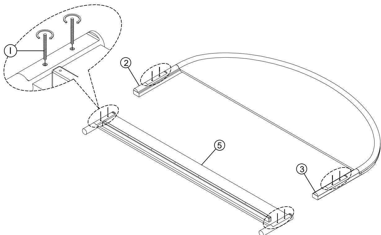
Attach the Hanger Bolts (I) to the Left Headboard Leg (2), Right Headboard Leg (3), and Footboard (5).
