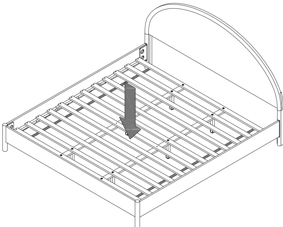
Place the assembled Slat Roll (4) Center Support Bar (7) and Support Leg (6) onto the Side Rails.
