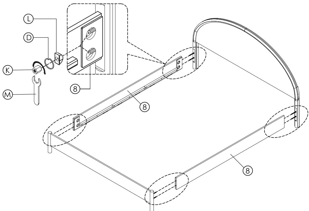
Assemble the Headboard and Footboard to the Side Rails (8) using Hex Nuts (K), Spring Washers (D), and Half Moon Washers (L) to secure the Headboard, Side Rails, and Footboard together. Tighten all nuts with the Open Wrench (M).
