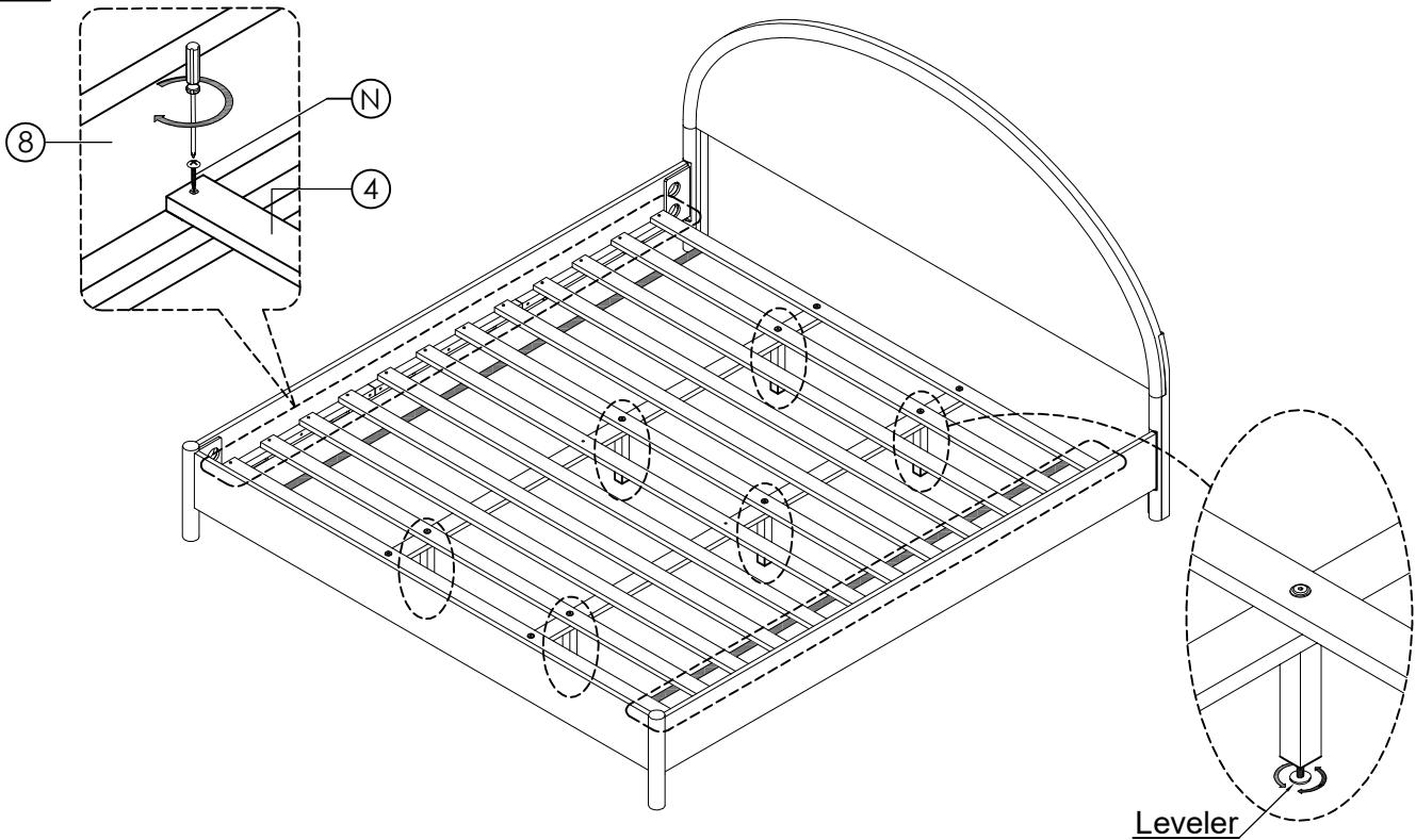
Use Screws (N) to secure the Slats Roll (4) to the Side Rails (8). You may adjust the leveler at the bottom of the Support Leg (6) to balance it with the floor.
