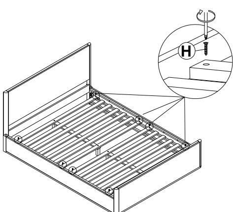
Lay the bed slats (P7) between the side rail (P5) using hardware:
