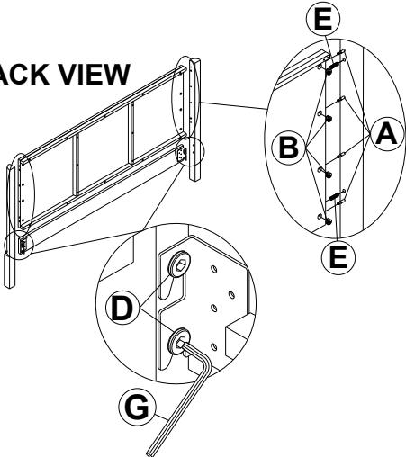
Attach the headboard bottom rail (P3) to the headboard post (P2) using hardware:
