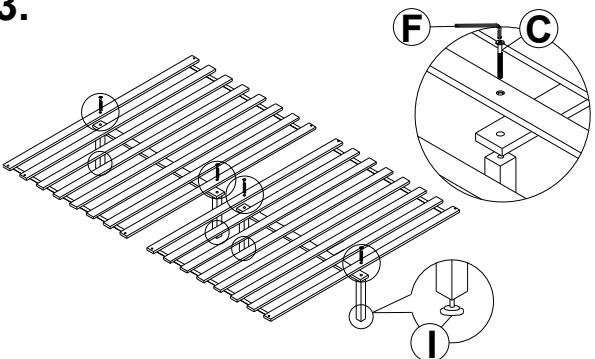
Fix the adjuster (I) to the support leg (P8) using hardware:
