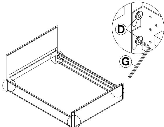
Attach the side rail (P5) to the headboard post (P2) and footboard (P4) using hardware:
