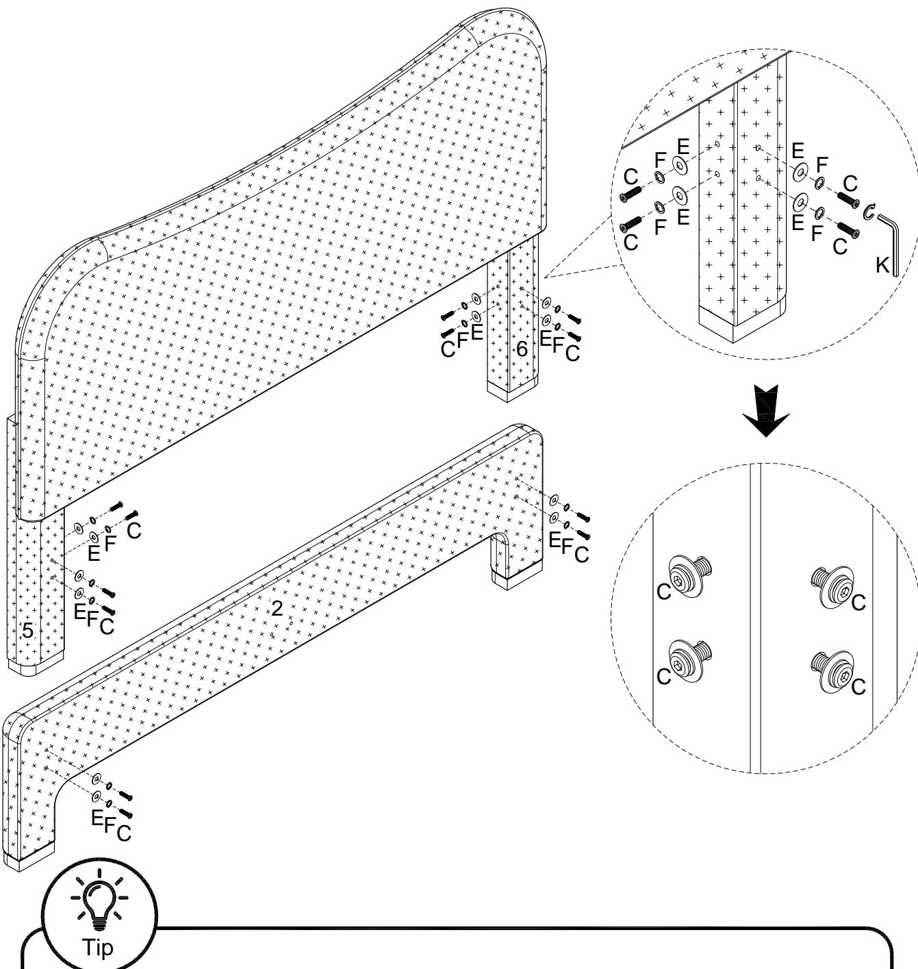
Do not tighten bolts / screws completely until all bolts / screws are lined up and inserted into holes. Tighten only to 50% for now.
