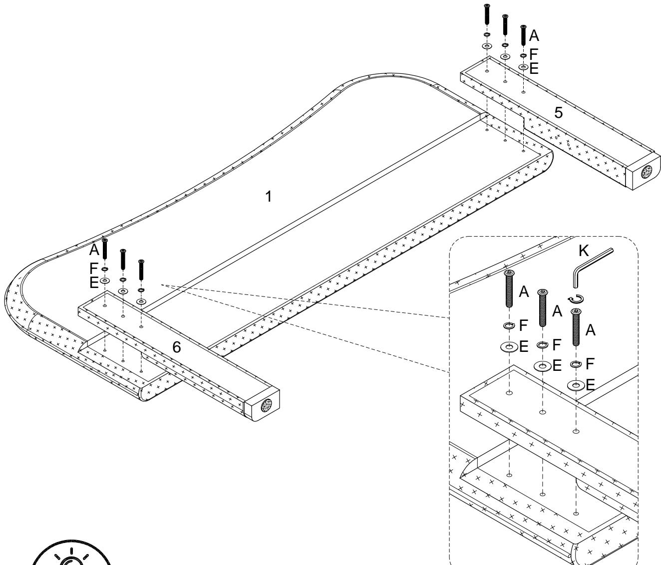
Do not tighten bolts / screws completely until all bolts / screws are lined up and inserted into holes. Tighten only to 75% for now.
