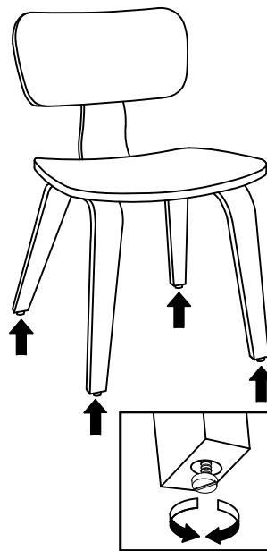
Turn clockwise or anti-clockwise to adjust leg leveller.
