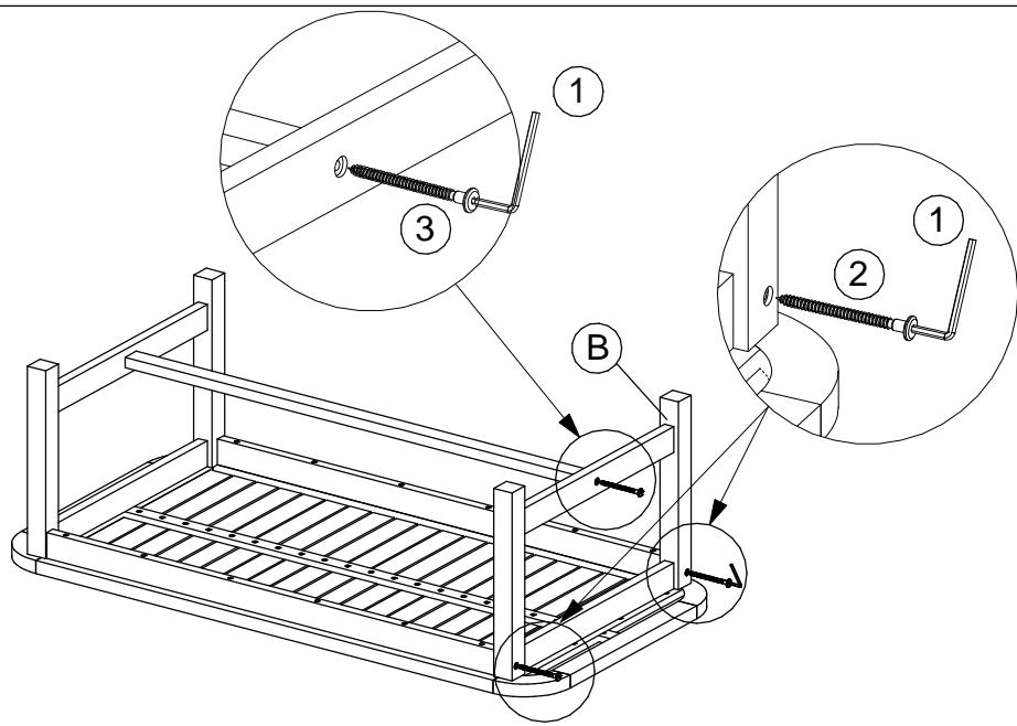
With assistance from your adult partners, attach Leg Panel (B) to Table Top (A) by using 2 Screws ( ) with Allen Wrench ( ) to secure as shown above.
