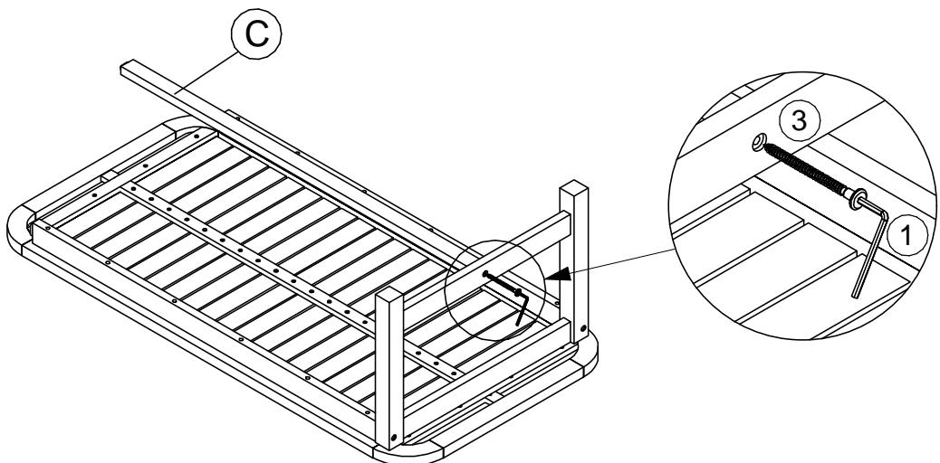
With assistance from your adult partners, attach Support Bar (C) to Leg Panel (B) by using 1 Screw ( ) with Allen Wrench ( ) to secure as shown above picture.
