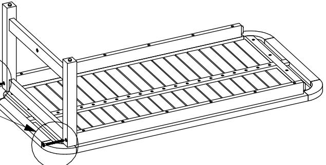
With assistance from your adult partners, position Leg Panel (B) and Table Top (A) as shown above picture. Attach Leg Panel (B) to Table Top (A) by using 2 Screws ( ) with Allen Wrench ( ) to secure as shown above.
