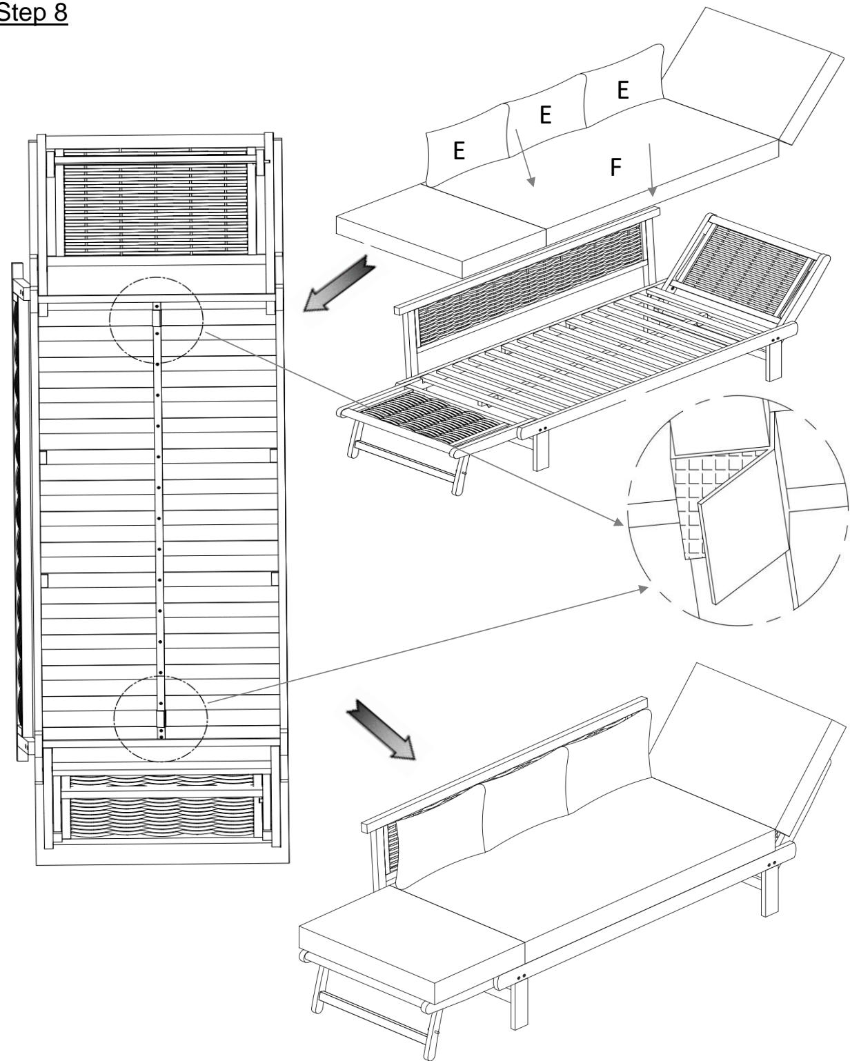
Place Seat Cushion (F) by affix the Magic Tape Straps on the seat slats of Seat Panel (B) as shown above, then place Back Cushions (E) onto Seat Cushion (F) as shown above.
