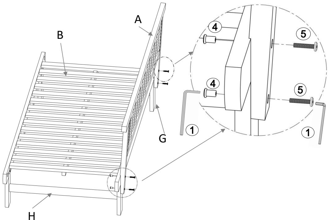
With assistance from your adult partner, attach Backrest Panel (A) to both Seat Panel (B), Left Leg (G) and Right Leg (H) by using Bolts (5) and Sleeve Nuts (4) with Allen Wrenches (1) as shown above.
