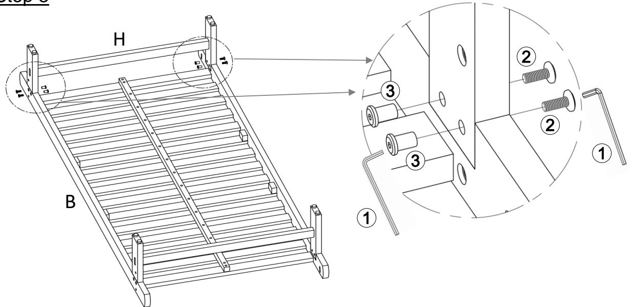
With assistance from your adult partner, attach Right Leg (H) to Seat Panel (B) of the assembled part in Step 2 by using Bolts (②) and Sleeve Nuts (③) with Allen Wrenches (①) as shown above.
