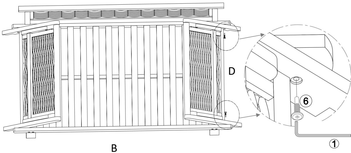
With assistance from your adult partner, attach Right Armrest Panel (D) to Seat Panel (B) by using Bolts (⑥) with Allen Wrench (①) as shown above. **DO NOT fully tighten the Bolts.**
