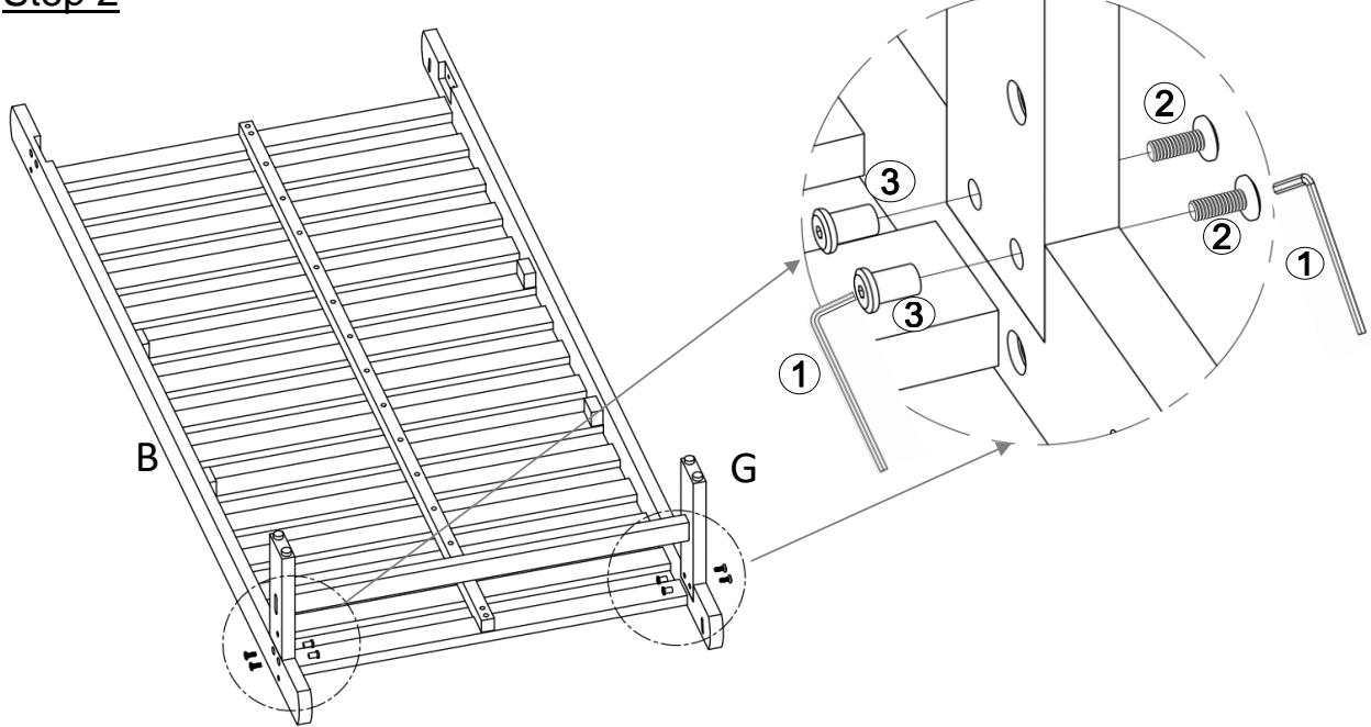
With assistance from your adult partner, place the Seat Panel (B) facing down then attach Left Leg (G) to Seat Panel (B) by using Bolts (②) and Sleeve Nuts (③) with Allen Wrenches (①) as shown above.
