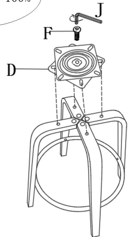
Finally tighten all screws to a depth of 100%.
