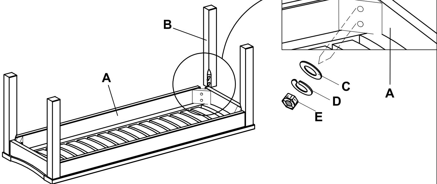
Insert the leg frame (B) into each corner of backless bench (A).
