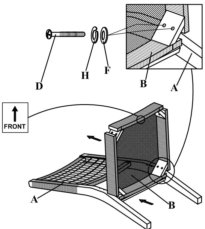
Attach the seat (B) to Back rest (A). Ensure the seat (B) align to the matching holes. Insert the small washer (F), spring washer (H) and 2" bolts (D) to the holes as shown in the diagram above. Adjust the bolts to the right position before screwing. Do not fully tighten the bolts yet.
