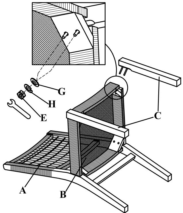
Attach the legs (C) into the seat (B). Secure it with big washer (G), spring washer (H) and nut (E). Tighten all bolts and nuts using screwdriver and wrench.
