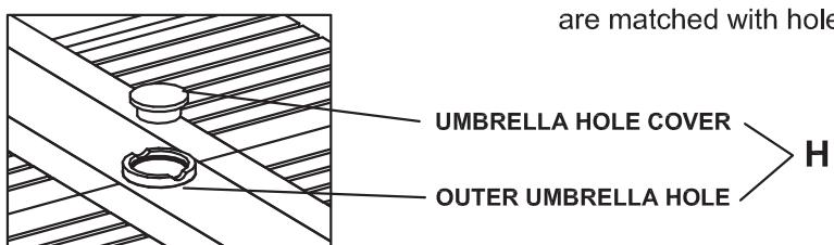
Put the umbrella hole plug (H) into hole of table top (A) as diagram shown.
