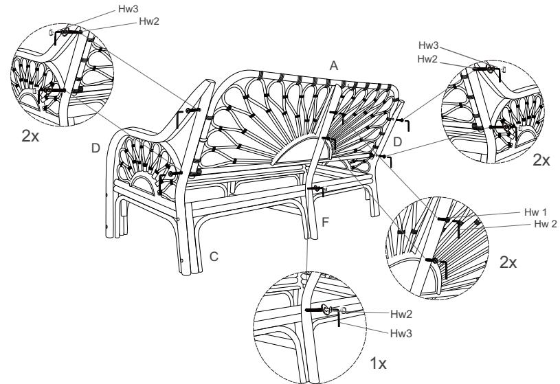
Place the Seat Frame (B) on the assembled frame. Place the Cushion (G) on the Seat Frame (B). Insert the Hole Covers (HW4) Press with small hammer make sure to apply all the holes cover properly.
