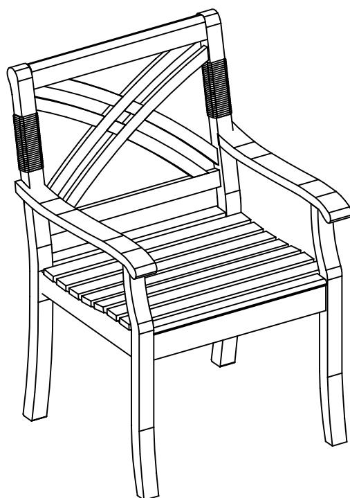
Turn the chair up right. Next, apply glue (K) to the holes both arms (D1&D2), next attach arms (D1&D2) to the backrest (A) and leg frame (B1&B2). secure using 2" screws on leg frame (B) and 1 3/4" bolt from backrest (A). as shown.
