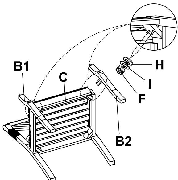
Attach the seat (C) into backrest (A), ensure the seat (C) align to the matching holes. insert the small washer (G), spring washer (I) and 1 3/4" bolts (E) to the holes as shown in the diagram above. Adjust the bolts to the right position before screwing
