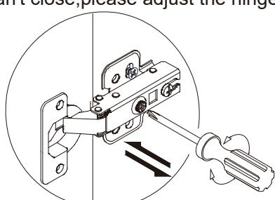
This is used to adjust the door panel in the left and right direction.
