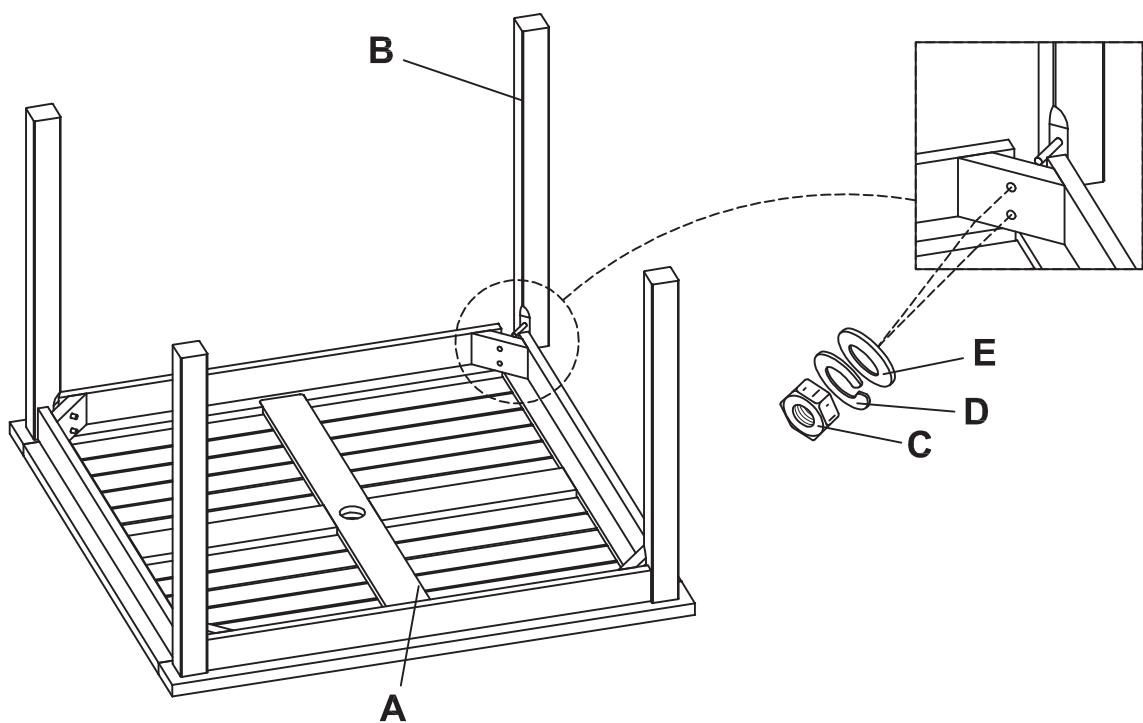
Attach the leg frame (B) into each corner of the top table (A).
