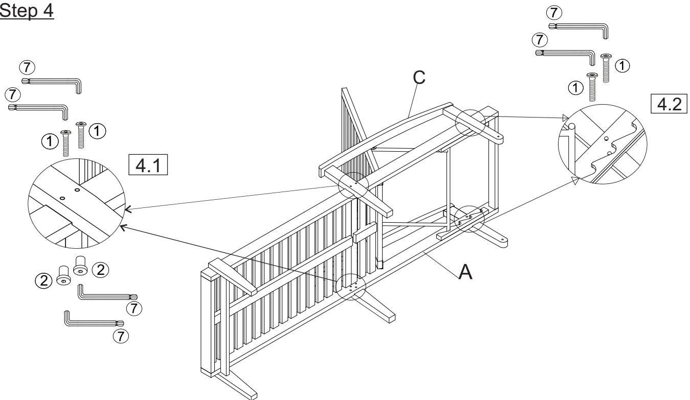
4.1) With the help of adult partner, attach 2 Left Leg Panel (C) to Foldable Seat Panel (A) using Bolts (①) and Sleeve Nuts (②) with Allen Wrench (⑧).
