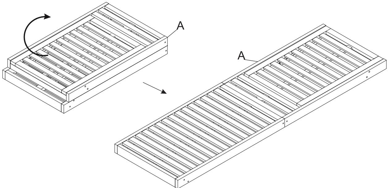
Unfold the Foldable Seat Panel(A) as indicated by the arrows.
