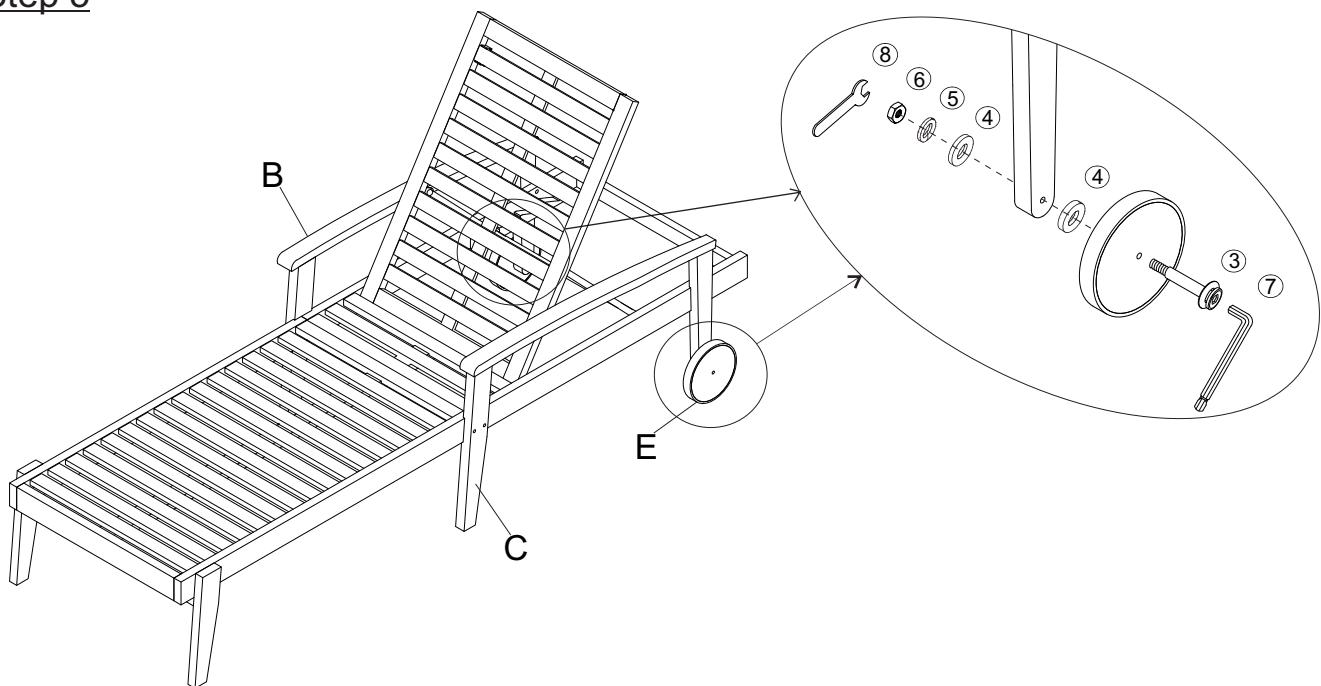
With the help of your adult partner, attach Wheels (E) to Right Leg Panel (C) using Wheel Bolt (3), Washers (4), Washers (5), Spring Washers (6) and Nuts (7) with Allen Wrench (8) and Wrench (9) in the sequence as shown above. Repeat the same process with remaining Wheel (E) and the Left Leg Panel (B). **Do not fully tighten the Bolts.**
