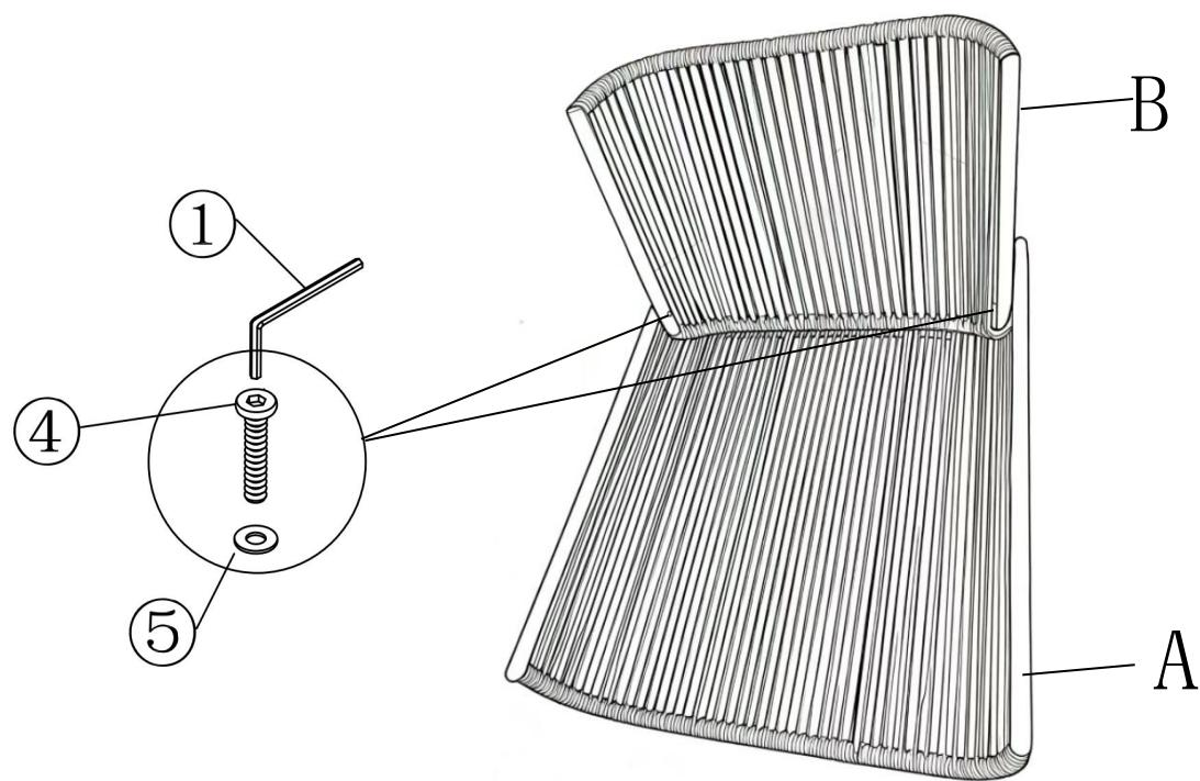
Attach the Seat Panel (B) to Backrest (A) using Bolts (④) and Washer (⑤) with Allen Wrench(①).
