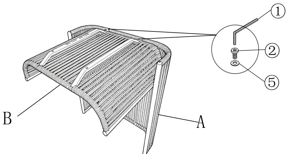
Using Bolts(②) and Wahser (⑤) with Allen Wrench (①) to connect the Seat Panel (B) and Backrest (A).
