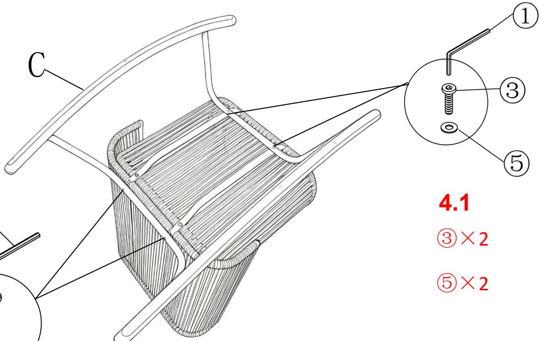
**4.1** Using Bolts (③) and Wahser (⑤) with Allen Wrench (①) to connect the Rocker Part (C) to the Seat Panel (B) as shown above.
