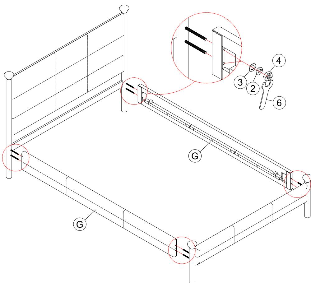
Attach the Side Rail (G) to the assembled Footboard from Step 4 and headboard from Step ⑤. by using spring washers ②, flat washers ③, Hexagonal nut ④ with Open wrench ⑥
