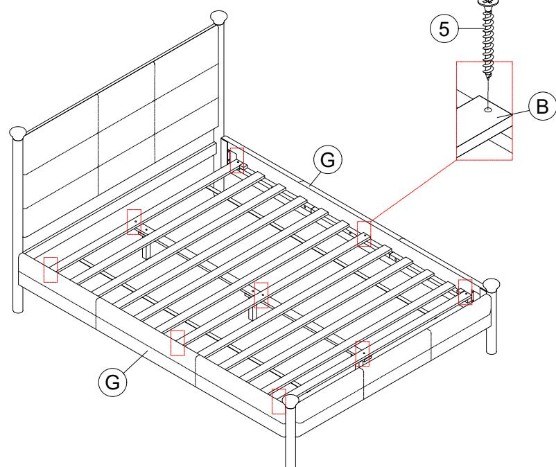
Place the Center Support Rails(H) and Slat (B) to the middle of the Bed Frame as shown above. Align the mounting position on Slat (C) to Center Support Rails(H) and Side Rails (G) ,then attach them together by using Screw (5) with Screwdriver(unprovided).
