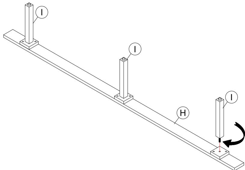
Attach the Support Leg (I) to the Center Support Rail (H) as shown.
