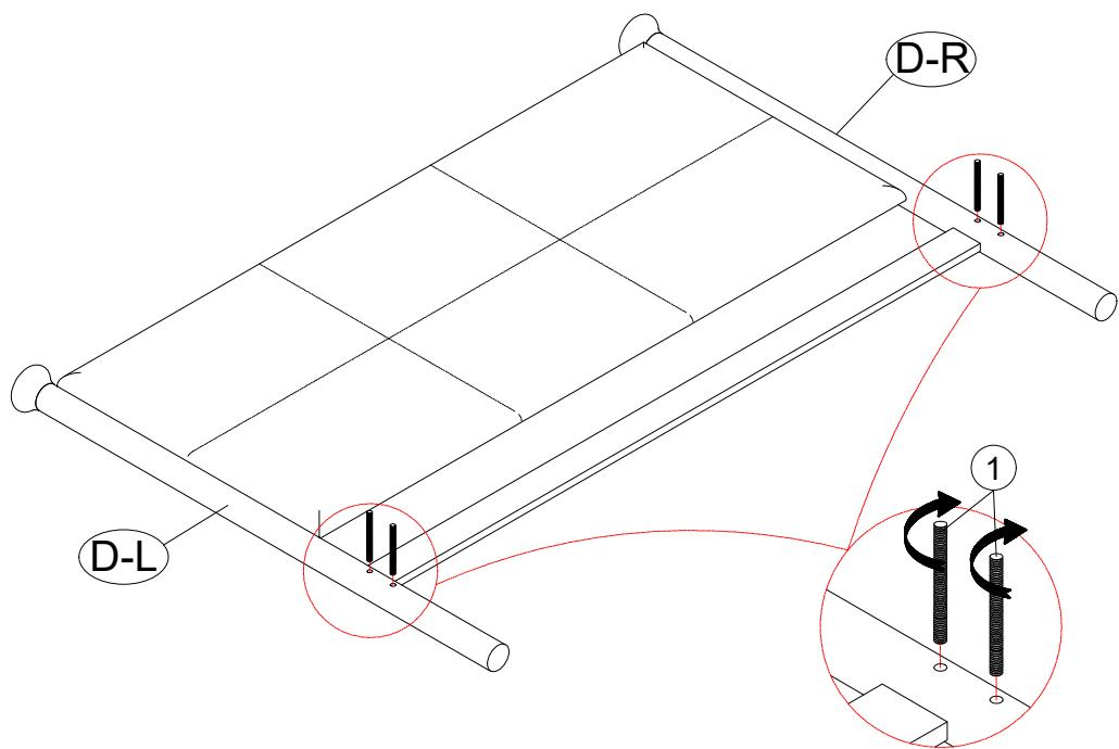
Screw the Insert Bolt ① to the Headboard Legs (D-L) & (D-R)
