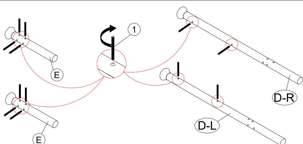
Screw the Insert Bolt ① to the Footboard Legs (E) and Headboard Legs (D-L) & (D-R)
