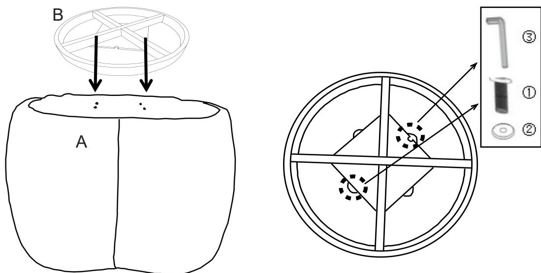
Rotate the base to align with the holes as the picture.
