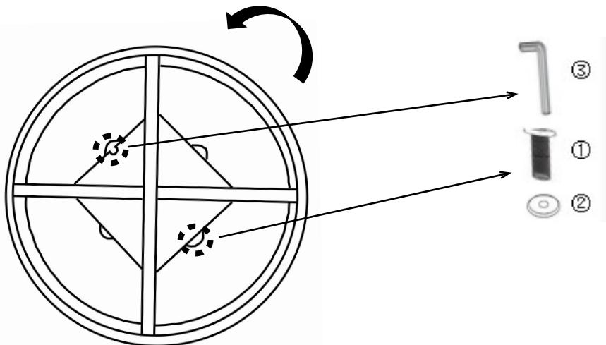
Rotate to align the remaining screw holes for installation.
