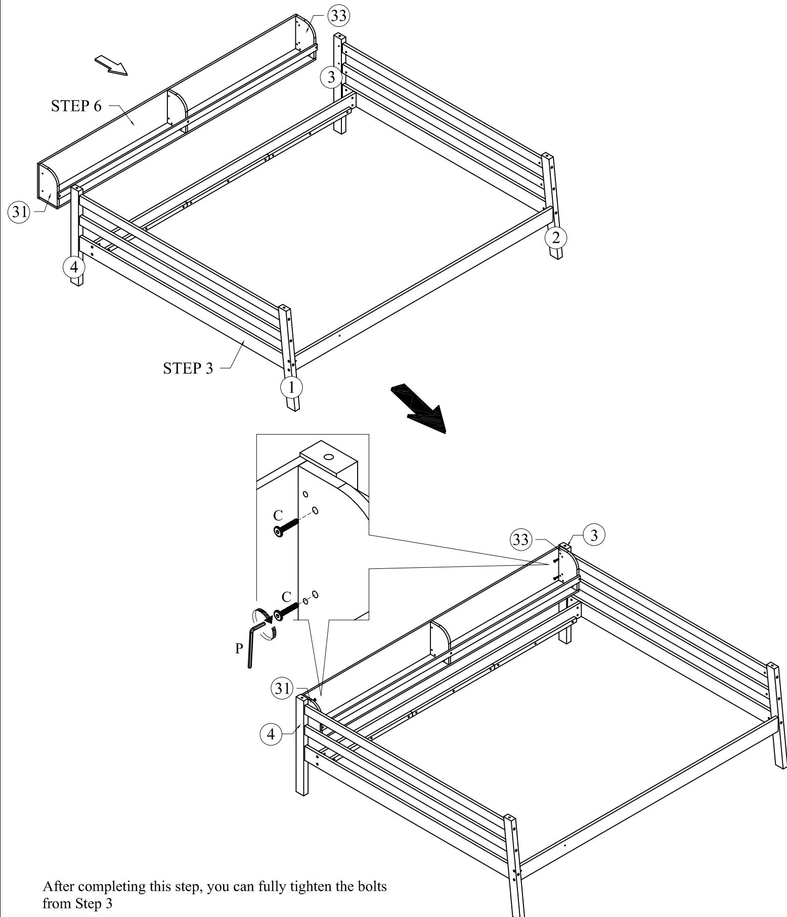
After completing this step, you can fully tighten the bolts from Step 3
