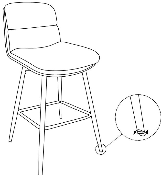
Remark: You can adjust leveling feet for balance.
