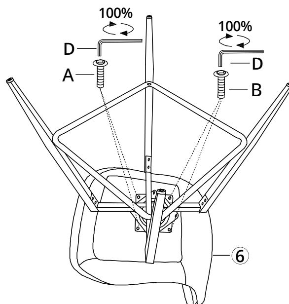
Remark: Install the 2 Bolts B on the holes near the backrest side.
