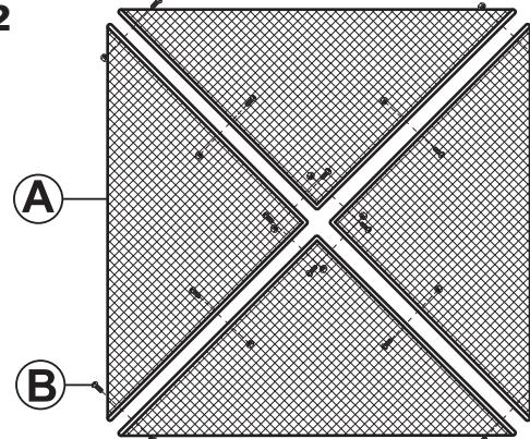
Secure screen panels (A) by hand-tightening M6x12mm Bolt Sets (B). Finish tightening all hardware.
