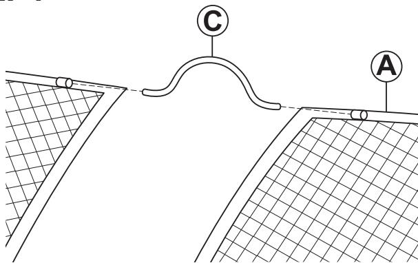
Install Handle (C) between retaining brackets on Screen Panels (A).
