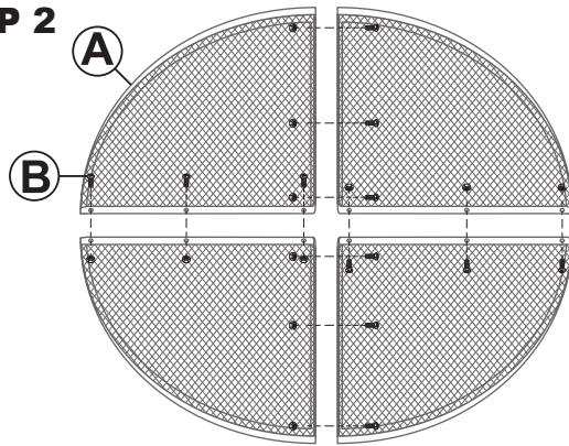
Secure screen panels (A) by hand-tightening M6x12mm Bolt Sets (B). Finish tightening all hardware.
