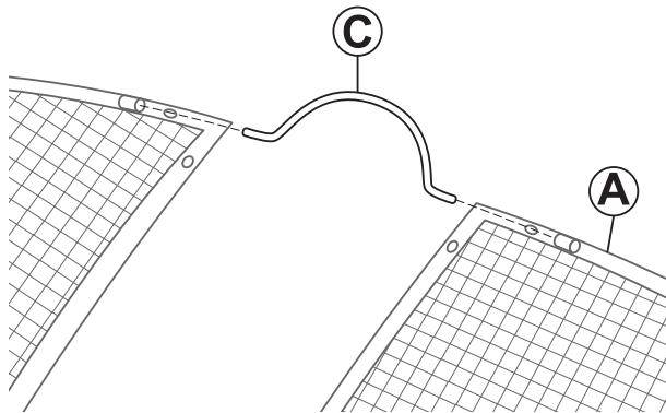
Install Handle (C) between retaining brackets on Screen Panels (A).
