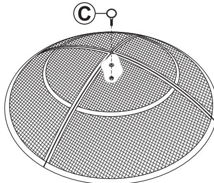
Install Handle Set (C) in the center of the screen. Finish tightening all hardware.
