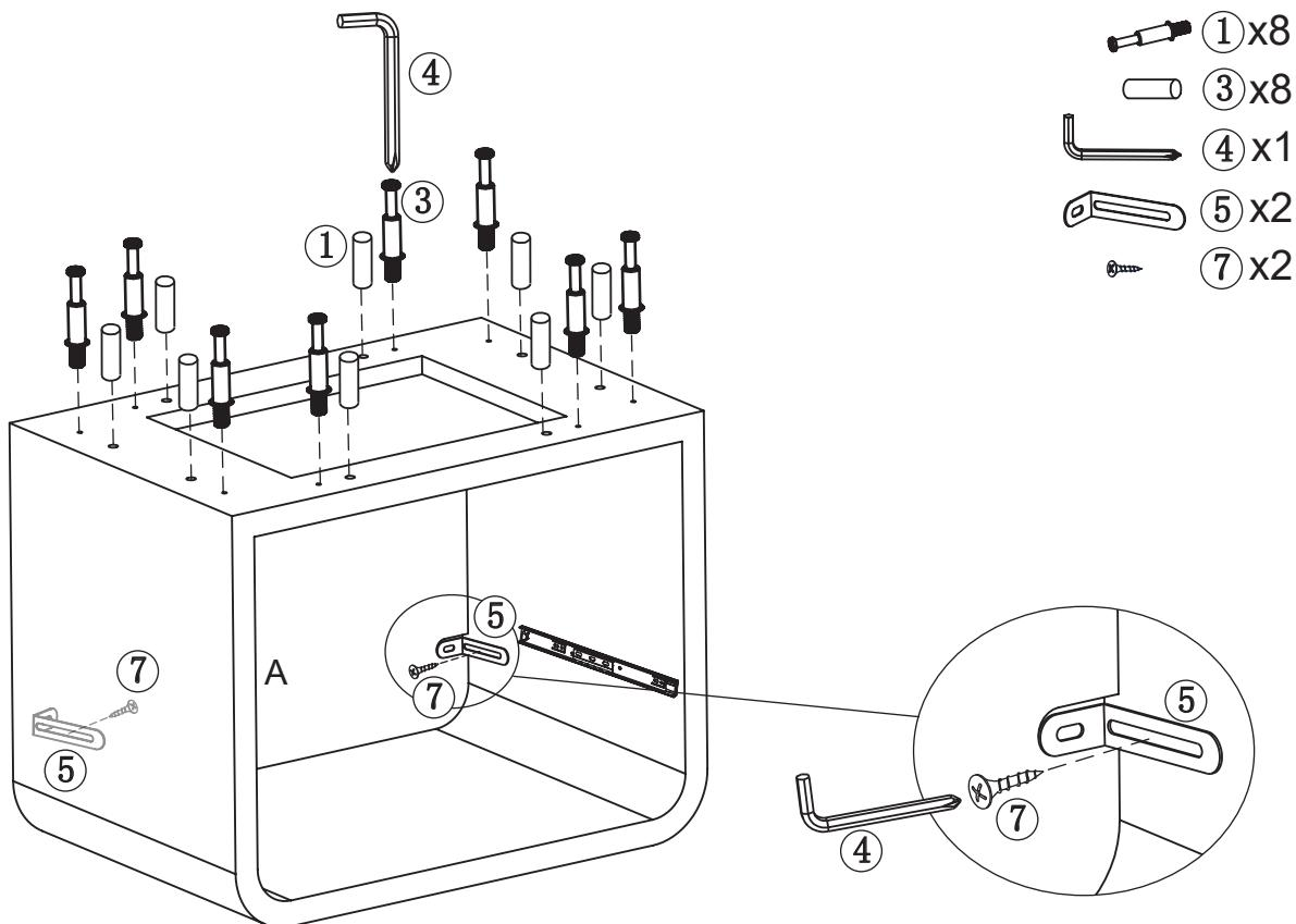
Attach cam bolt(①) and dowel(③) to the top panel (A) using I-type hexagon wrench(③). Attach the long side of anti-tipping sheet iron ( ⑤ ) connected to the top panel(A) with screw( ⑦ ) using I-type hexagon wrench (④).
