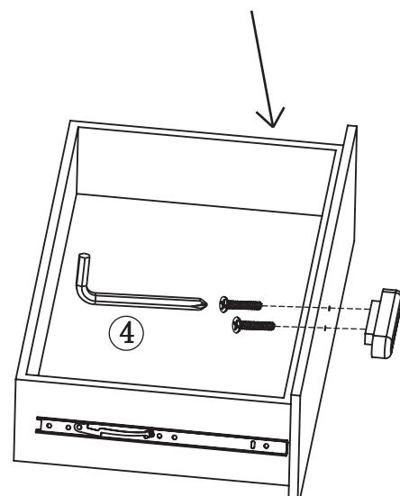
Lock the handle outside the drawer using I-type hexagon wrench (④).
