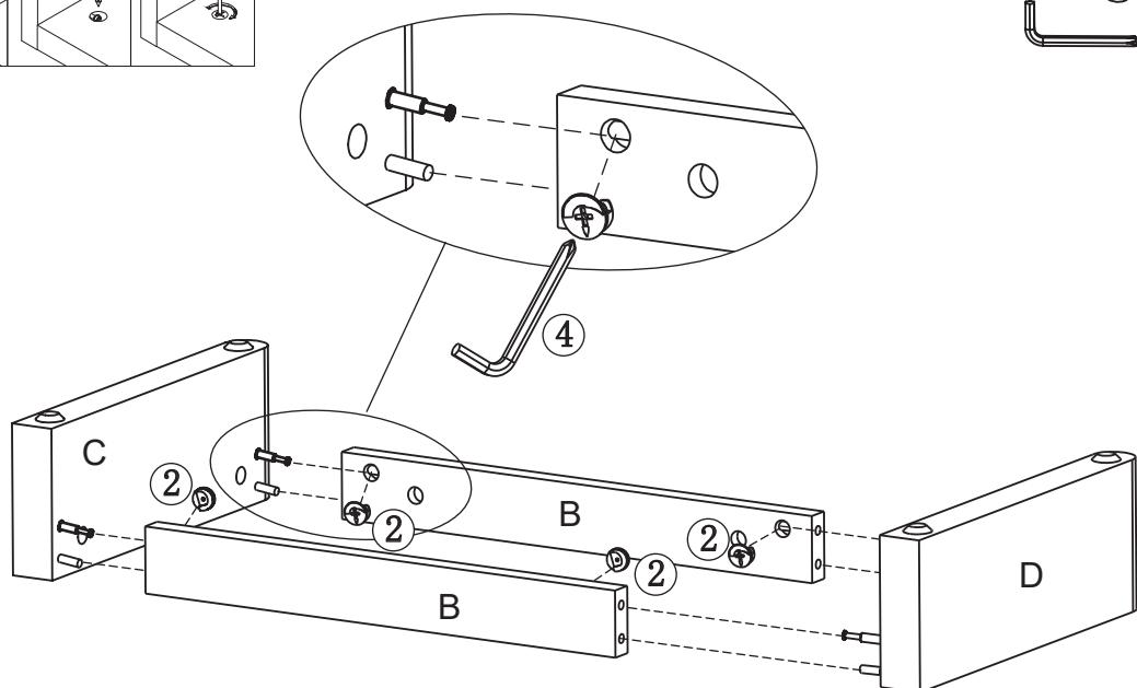
Attach the left leg (C) and the right leg (D) to the stick (B) with cam nut (2) using I-type hexagon wrench (4).
