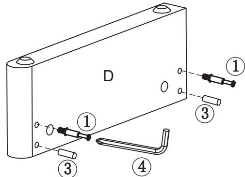
Attach cam bolt (1) and dowel (3) to the left leg (C) and the right leg (D) using I-type hexagon wrench (4).
