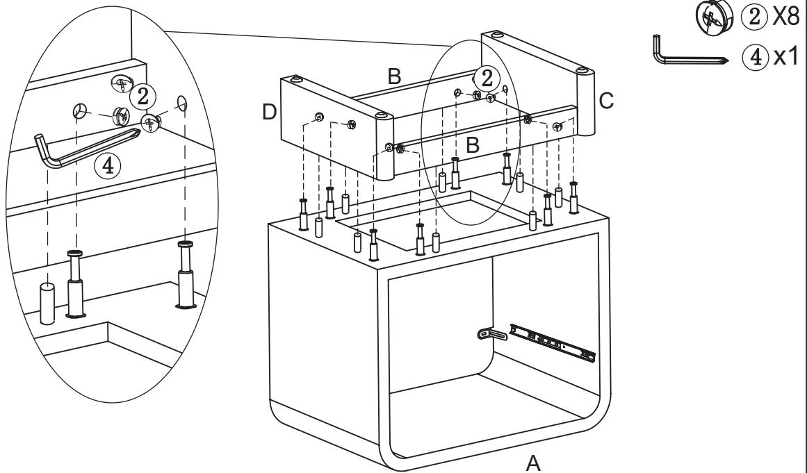
Attach the left leg (C), the right leg (D) and the stick (B) to the top panel (A) with cam nut(②) using I-type hexagon wrench (④).
