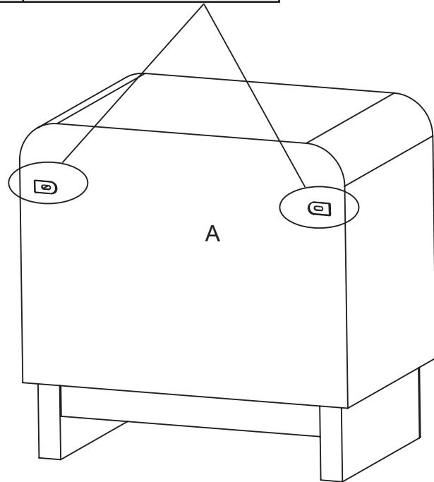
Screw the nut (⑥) into the wall. Install the short side of anti-tipping iron sheet (⑤) on the wall with screw( ⑧) using I-type hexagon wrench (④).
