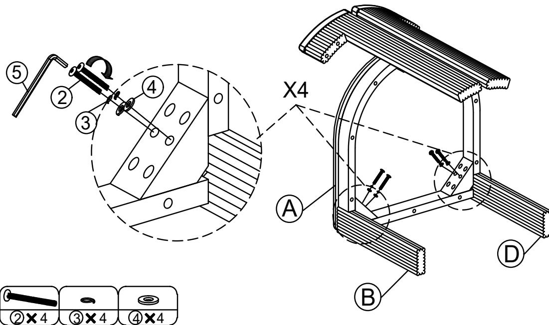
Step 3: Attach the two chair legs (B, D) to the chair frame (A) using bolts (2), washers (3), lock washers (4), and tighten securely with the Allen Wrench (5).
