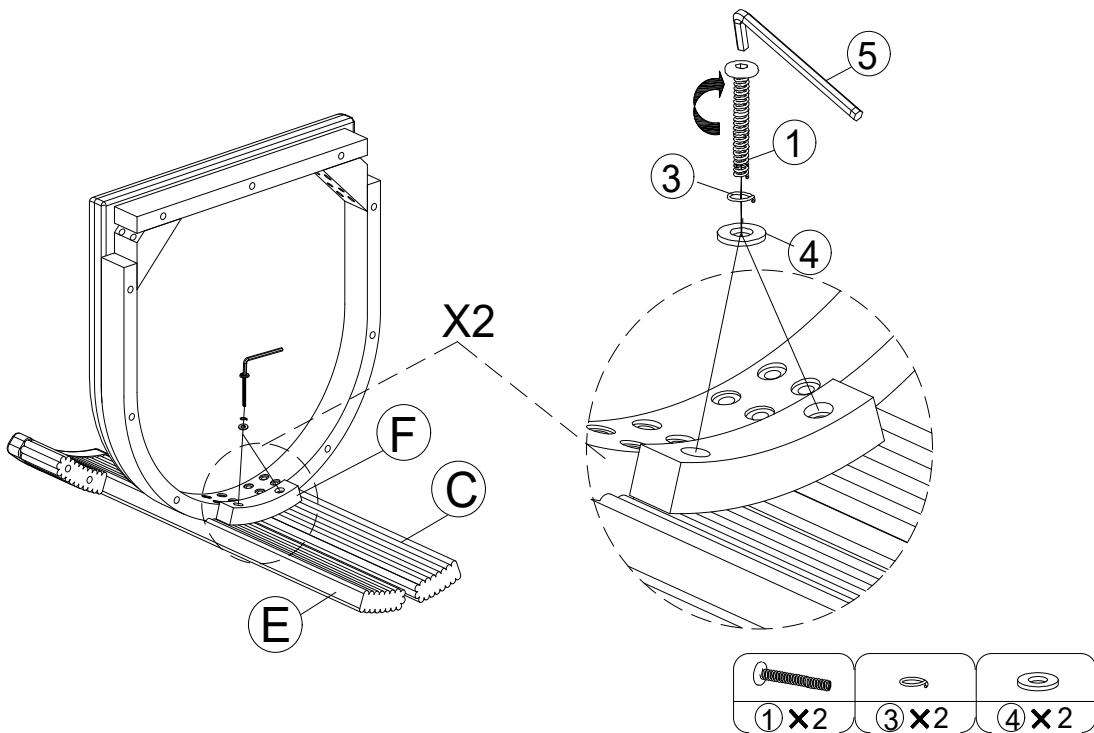
Step 2 : Attach the one chair back side rail (F) to the chair legs (C, E) using bolts (1), washers (3), lock washers (4), and tighten securely with the Allen Wrench (5).
