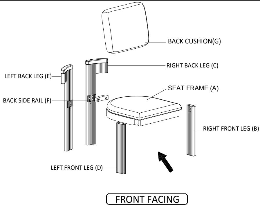
This chair has multiple parts and may require up to 15 minutes to assemble. The picture above provides an overview of the chair parts to help you visualize and understand each component. Please read through the instructions below to familiarize yourself with the parts and steps before assembly.
