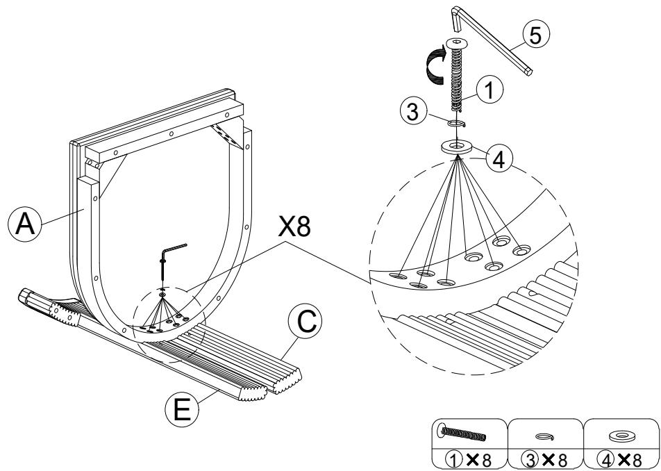
Step 1: Attach the two chair legs (C, E) to the chair frame (A) using bolts (1), washers (3), lock washers (4), and tighten securely with the Allen Wrench (5).
