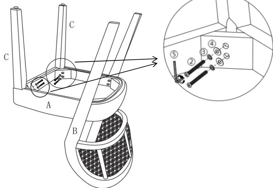
Place the Pack of Seat(A) and Back with legs(B) on the side of a table with the Seat(A) facing down, as seen in the picture.
