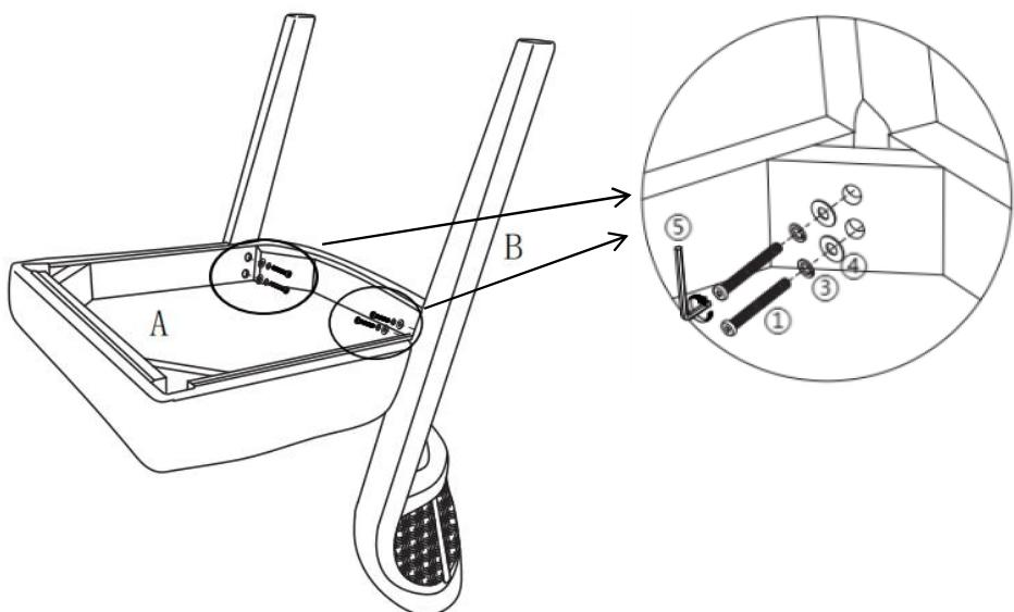
Place the Pack of Seat(A) and Back with legs(B) on the side of a table with the Seat(A) facing down, as seen in the picture.
