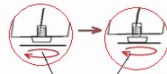
**Adjust Pre-installed Levellers height to achieve balance**
