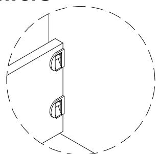
2. Once the pin is inserted correctly, flip the metal lever in the opposite direction to ensure the panels are firmly locked together.
