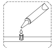
1: The provided glue is to secure wood dowels in place. When first inserting dowels, locate the appropriate hole for the dowel, place a small amount of glue in the hole and insert the dowel. Wipe away excess glue immediately.
