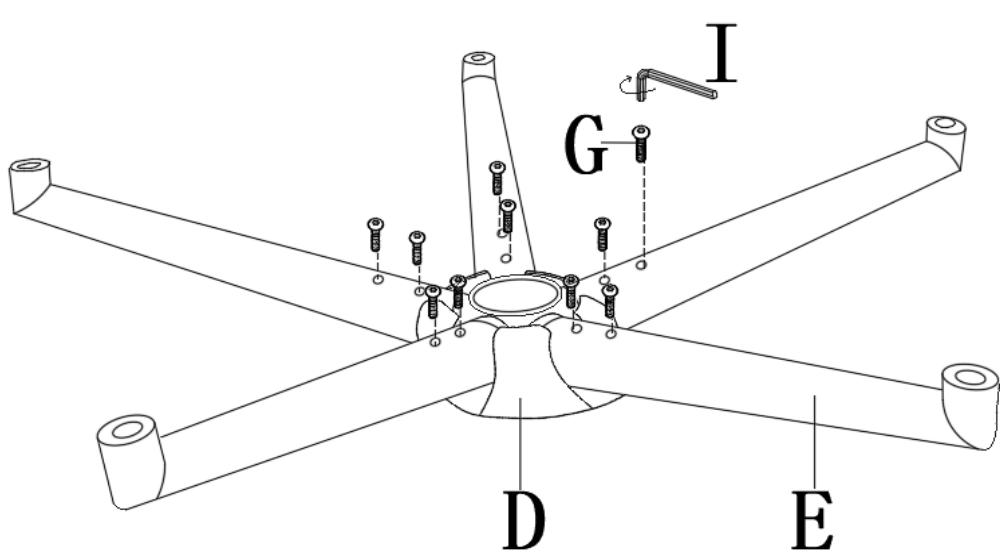
Finally tighten all screws to a depth of 100%.
