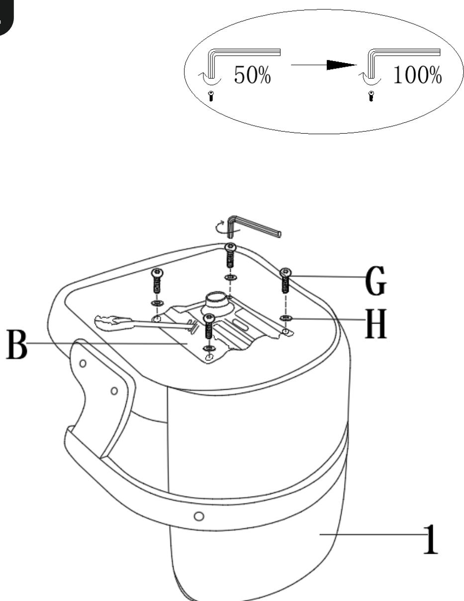
Finally tighten all screws to a depth of 100%.
