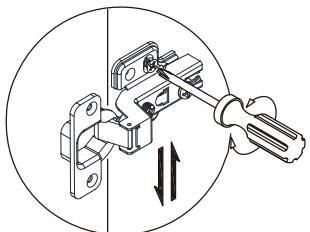
This is used to adjust the door panel in the up and down direction.
