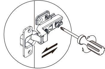
This is used to adjust the door panel in the front and rear.
