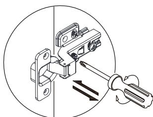
This is used to adjust the door panel in the left and right direction.
