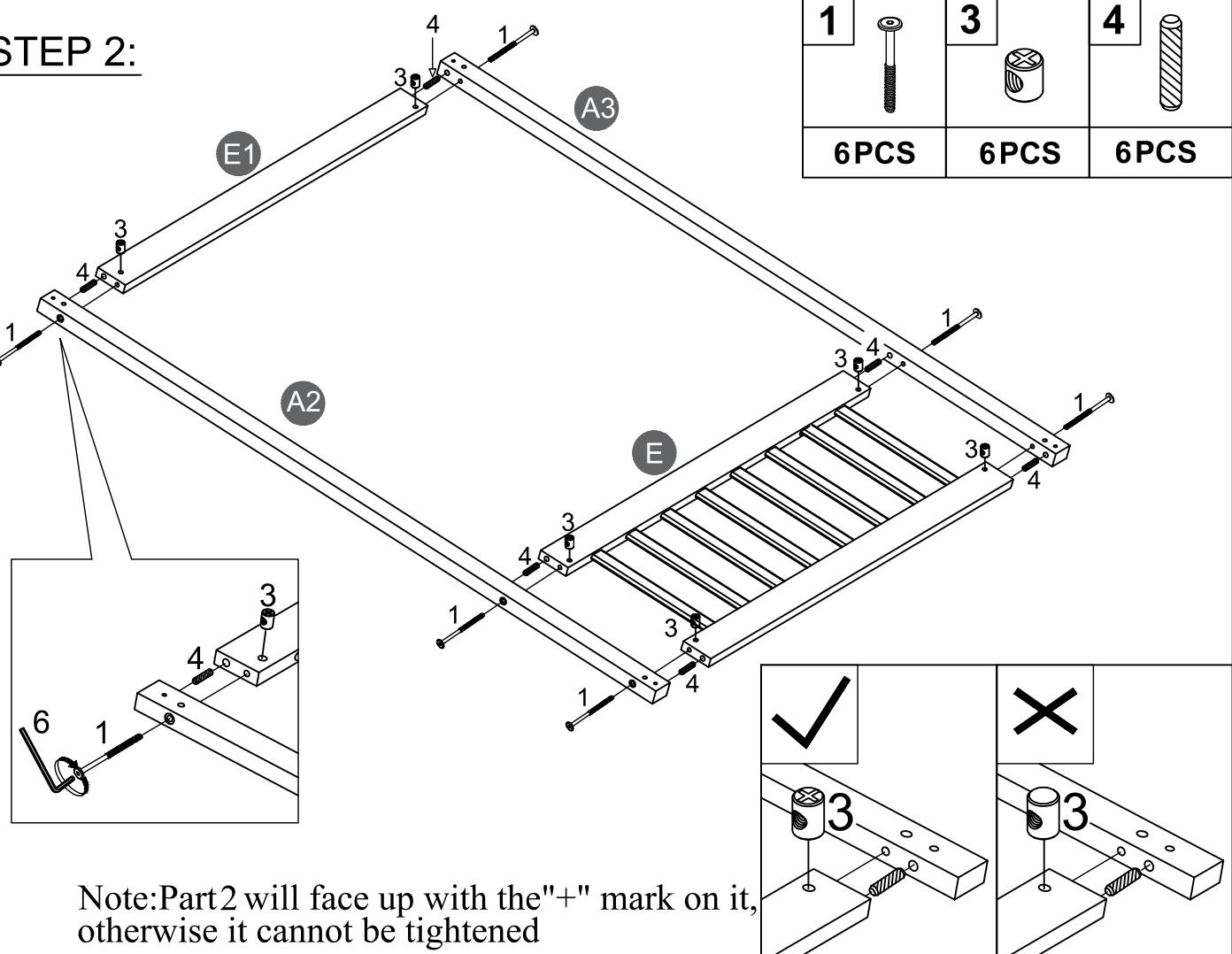
Note: Part 2 will face up with the "+" mark on it, otherwise it cannot be tightened
