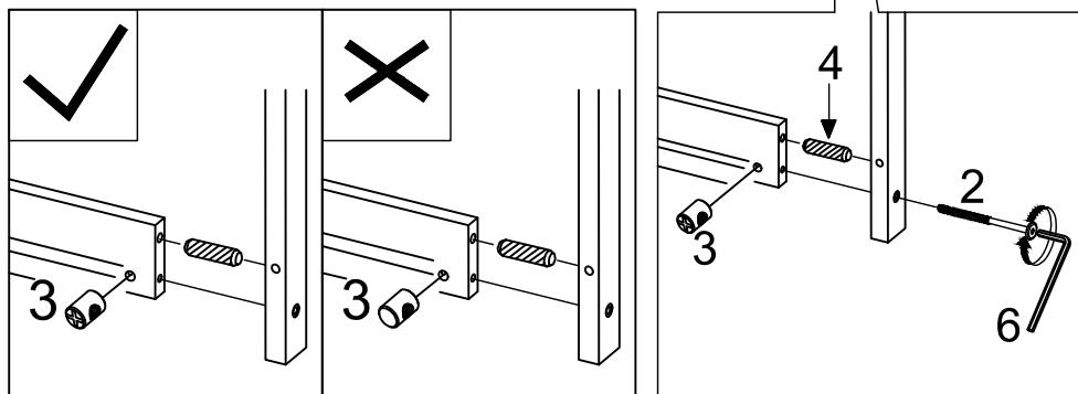
Note: Part 2 will face up with the "+" mark on it, otherwise it cannot be tightened
