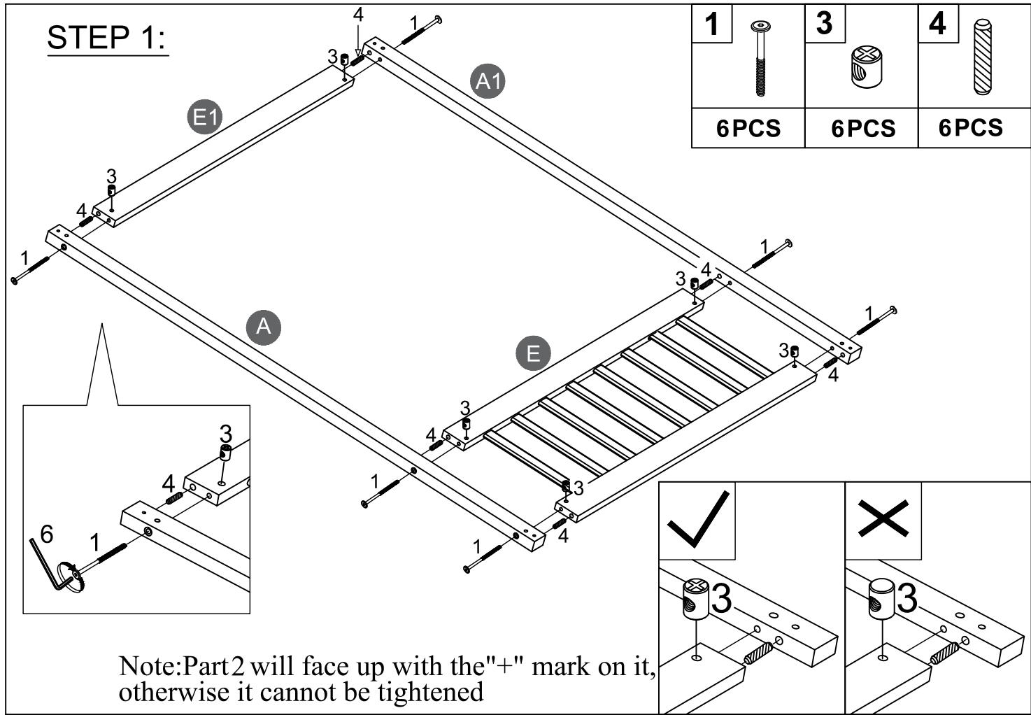
Note: Part 2 will face up with the "+" mark on it, otherwise it cannot be tightened
