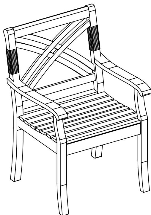
Turn the chair up right. Next, apply glue (L) to the holes both arms (D1&D2), next attach arms (D1&D2) to the backrest (A) and leg frame (B1&B2). secure using 2" screws (K) on leg frame (B) and 1 3/4" bolt (E) from backrest (A). as shown.
