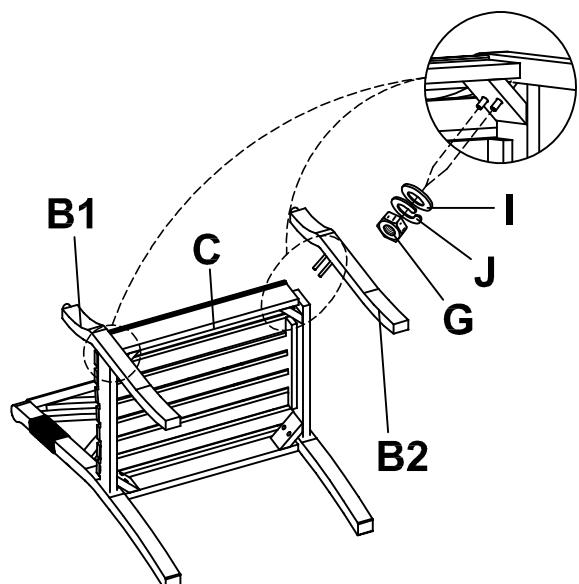
Attach the seat (C) into backrest (A), ensure the seat (C) align to the matching holes. insert the small washer (H), spring washer (J) and 2" bolts (F) to the holes as shown in the diagram above. Adjust the bolts to the right position before screwing
