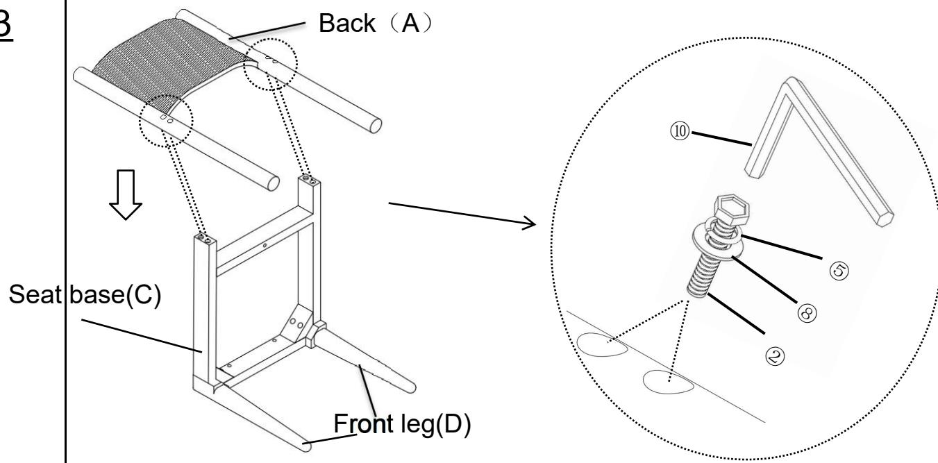
Attach the Back(A) into the mounting positions of the Seat base(C) using Bolts(②), Spring Washer(⑤) and Washer(⑧) with Allen Wrench(⑩).
