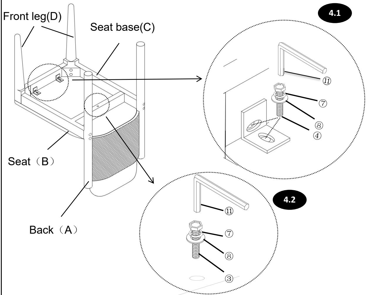
4.1) Attach the Seat base(C) and Seat(B) into the mounting positions of the angle iron(⑨) using Bolts(④), Spring Washer(⑦) and Washer(⑧) with Allen Wrench(⑪).
