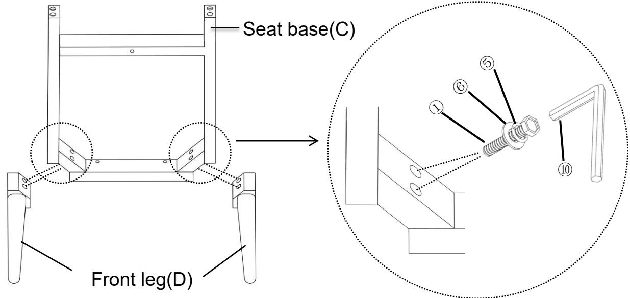
Attach the Legs(D) into the mounting positions of the Seat base(C) using Bolts(①) Spring Washer(⑤) and Washer(⑥) with Allen Wrench(⑩).
