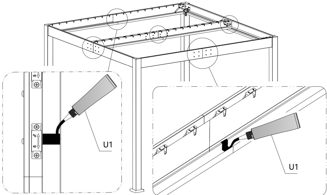
Wipe the inner side of each water tank joint clean and apply glass glue evenly.
