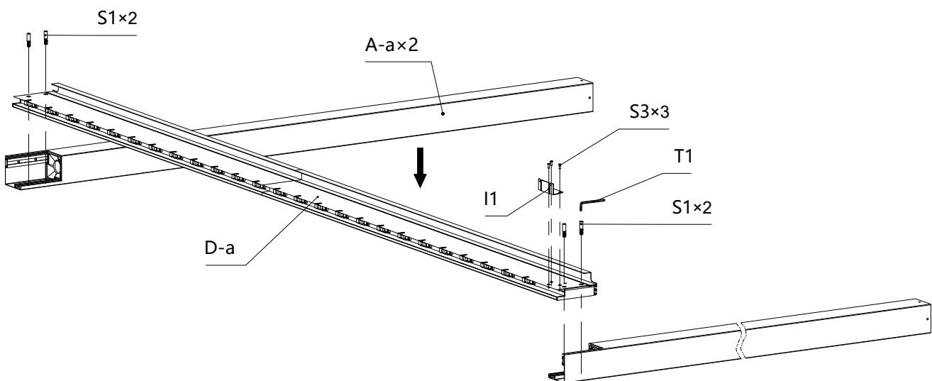
⚠ Connected by screws "S1", but don't tighten them at this step.
