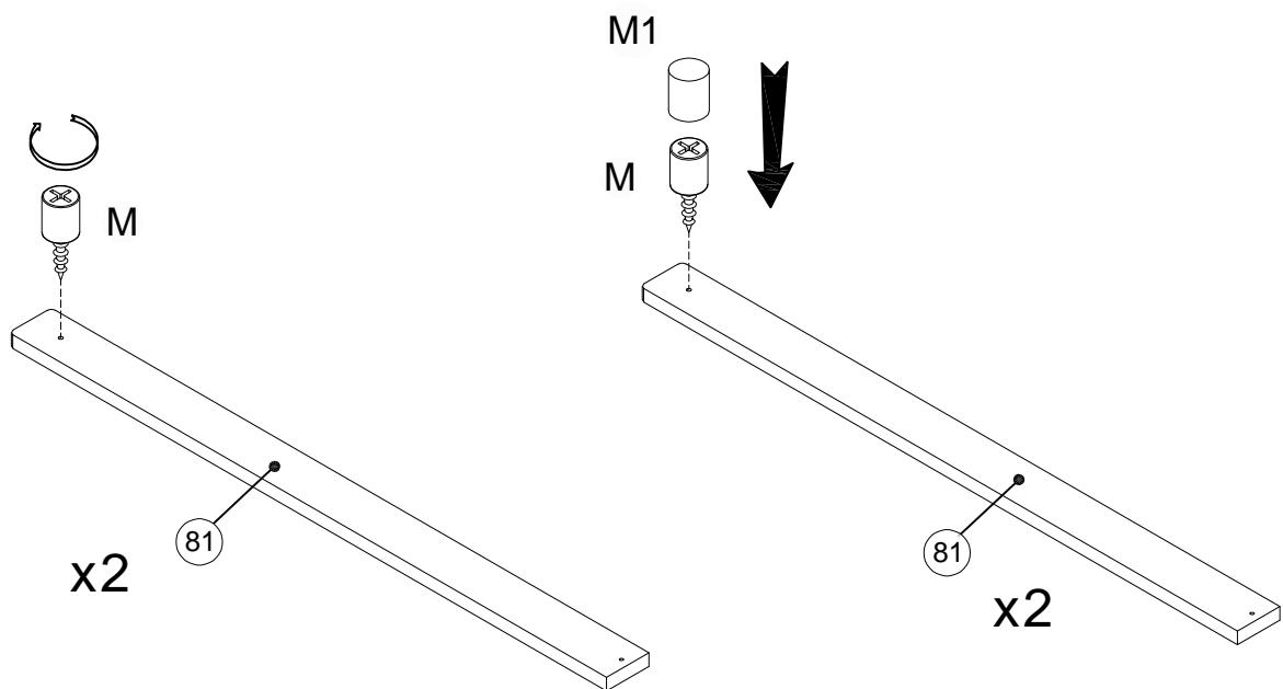
Assemble the stopper onto the slat bar, then fit the rubber cap on to reduce friction.
