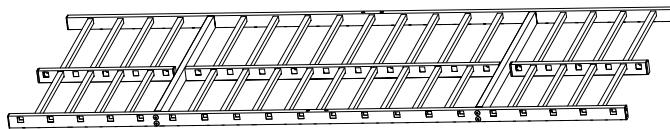
Step 10:This step requires two people to operate and install the semi-finished products of the previous step together. Use hardware A,B,C to connect #14,#16 together.
