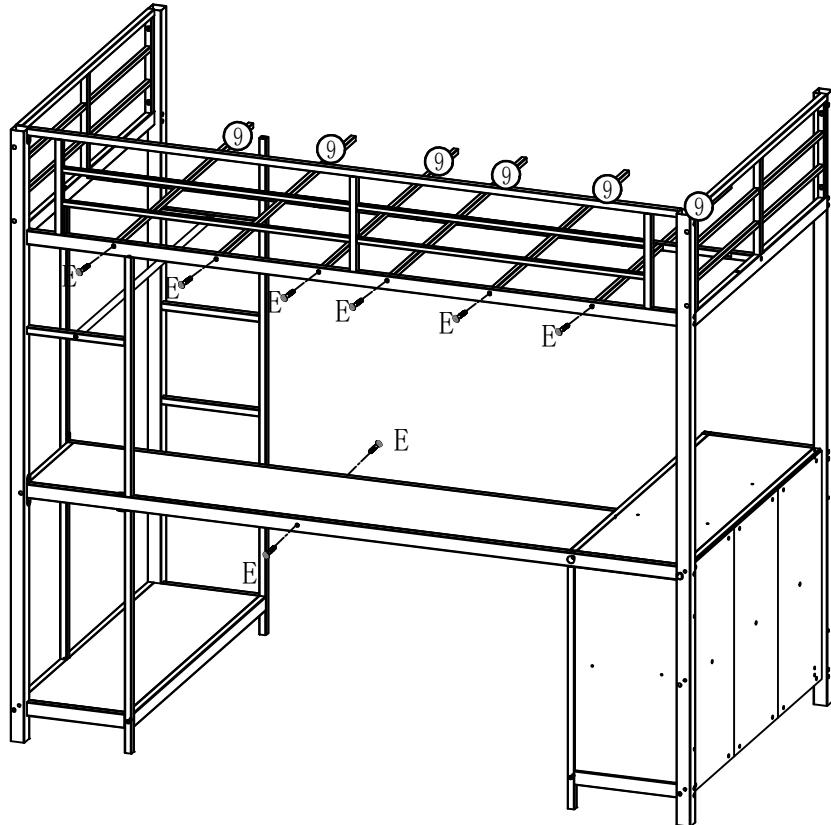
Step 9: Connect #10 and #6 to the previously installed components.
