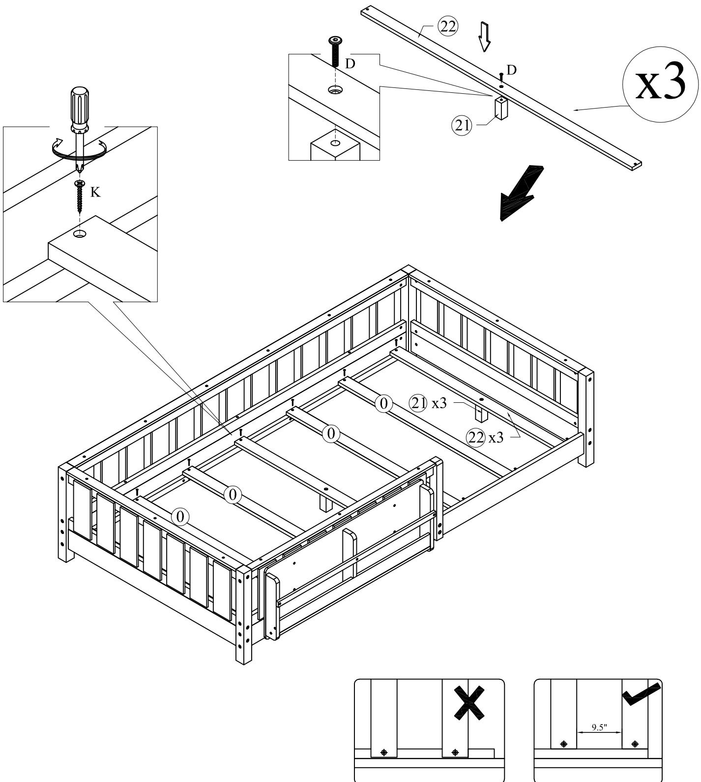
Check and fully tighten all bolts in the assembly steps to ensure a solid structure.
