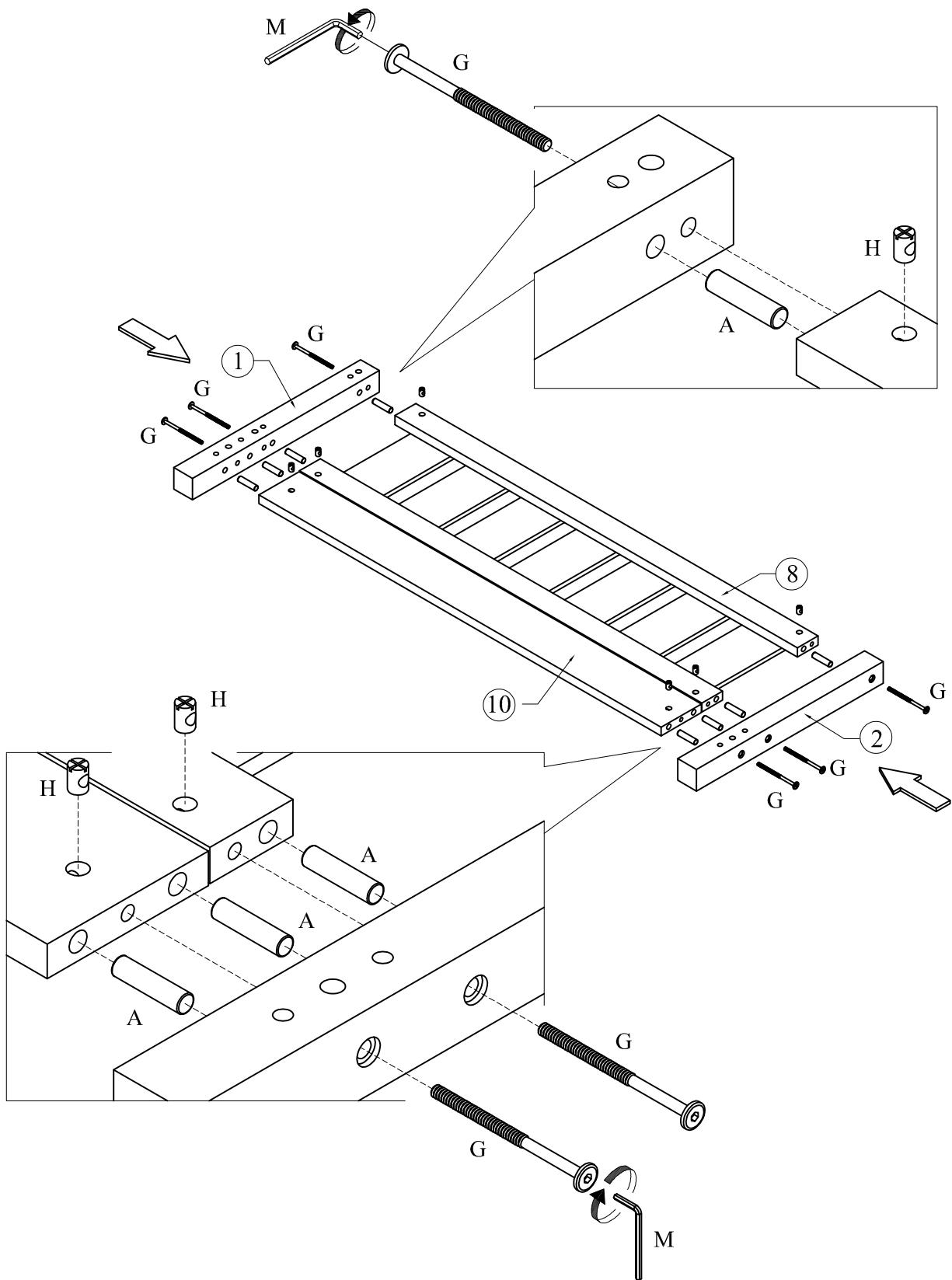
Note: Do not overtighten the bolts to ensure easier assembly in the next step.
