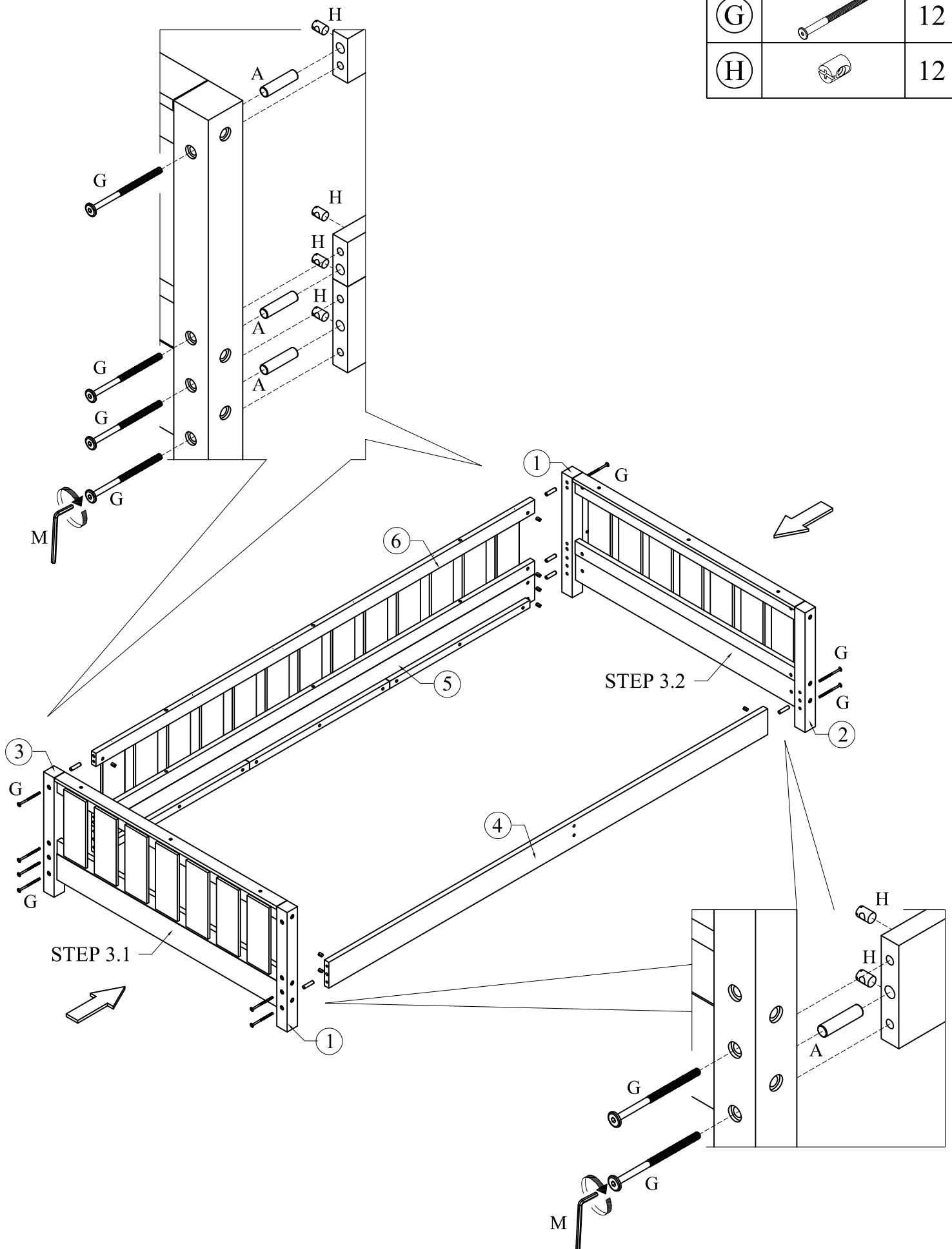
Note: Do not overtighten the bolts to ensure easier assembly in the next step.
