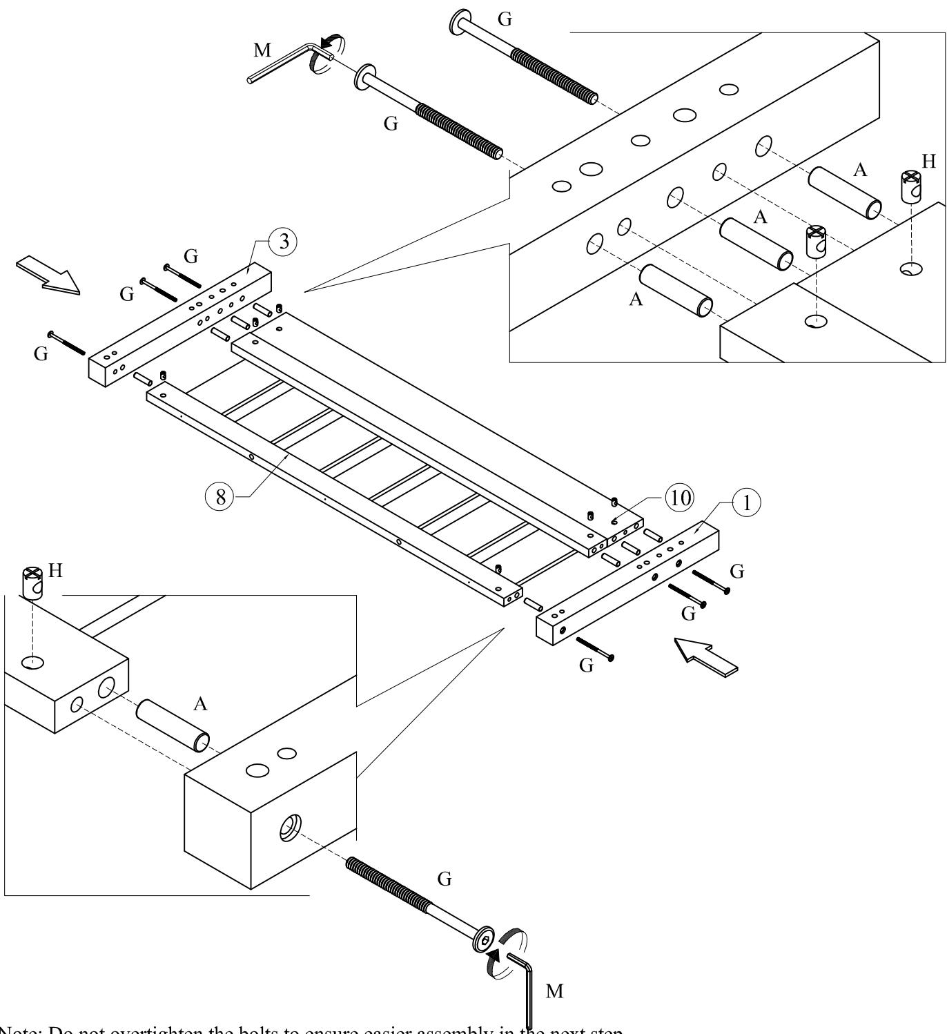
Note: Do not overtighten the bolts to ensure easier assembly in the next step.
