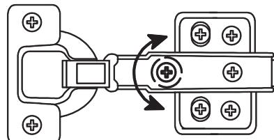
Loosen the side-to-side screws, then screw counter-clockwise to make the gap wider or clockwise to close any gaps.
