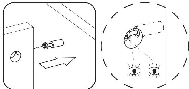
Next, you will notice the cam lock has a "C" shaped back. Commonly, an arrow on the front of the cam lock points in the same direction as the open section on back.
