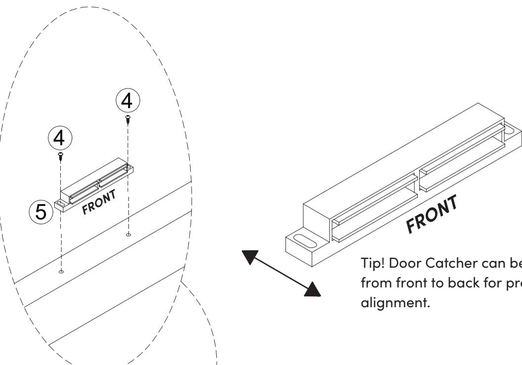
Tip! Door Catcher can be adjusted from front to back for proper door alignment.
