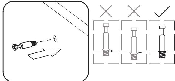
Next, you will fit the proper hole on the edge of the associated joining panel over the cam bolt.
