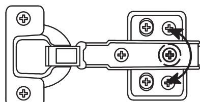
Adjust the in-and-out screws until the door is aligned with the side of the cabinet.
