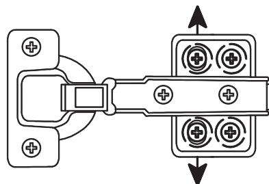
Loosen the height screws, then move the door up or down to make it level.
