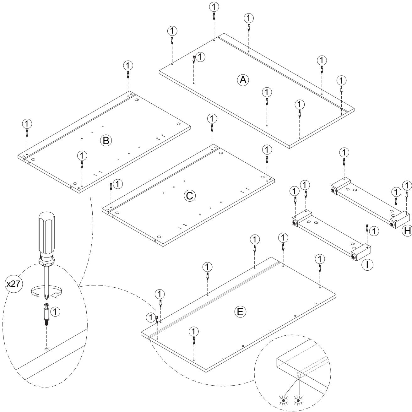
***The grooved side is on the bottom.***
