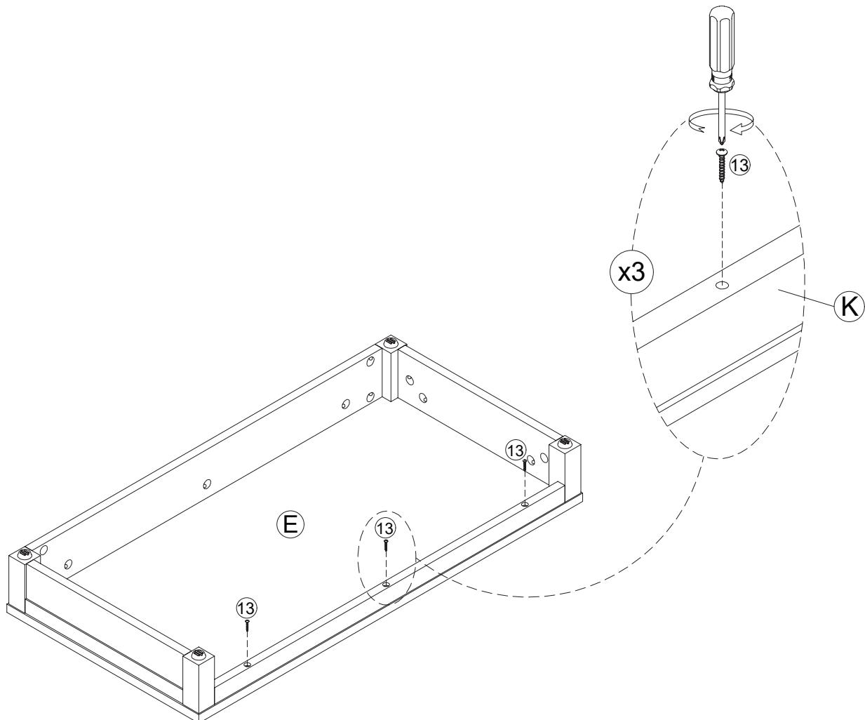
Please be careful not to use the wrong screw when installing Base Stretcher (Front) (K).
