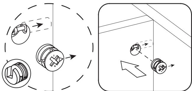
Using a screwdriver, you will turn the cam lock until it stops, usually at  $90^\circ$  or  $180^\circ$ . You will feel the panels pulling closer until they are secured.
